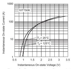
Fig. 7 - On-State Voltage Drop Characteristics
