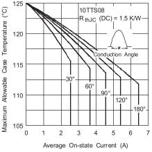
Fig. 1 - Current Rating Characteristics
