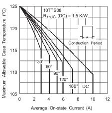
Fig. 2 - Current Rating Characteristics
