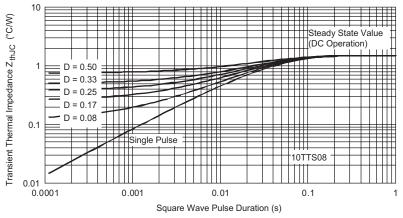
Fig. 8 - Thermal Impedance  $Z_{thJC}$  Characteristics
