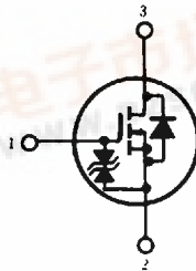
2SK408 1 Gate 2 Source 3 Drain
