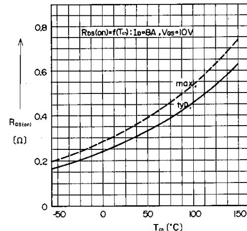
On State Resistance vs.  $T_{ch}$
