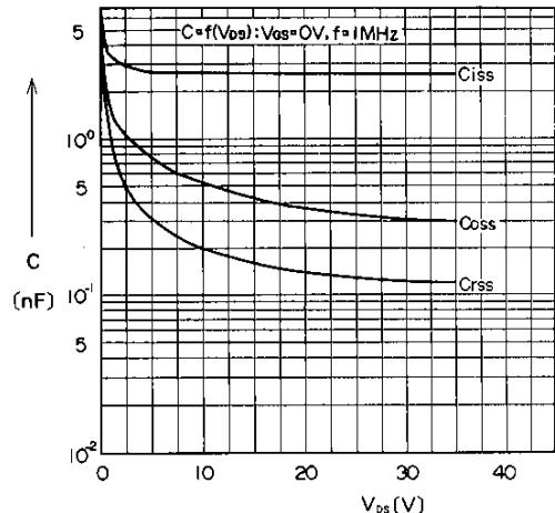
Typical Capacitance vs.  $V_{ds}$
