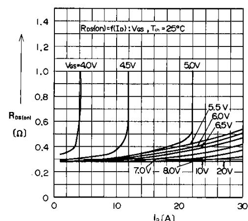
Typical Drain-Source on State Resistance vs.  $I_D$
