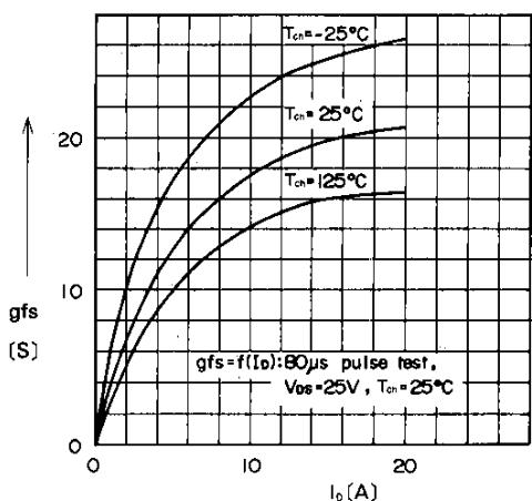
Typical Forward Transconductance vs.  $I_D$
