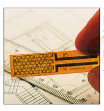
Heat Flow sensors allow precision measurements of heat transfer through any surface material. They are cemented onto a surface like strain gauges, and will give an accurate measurement of heat transfer using a DVM as an indicator.
