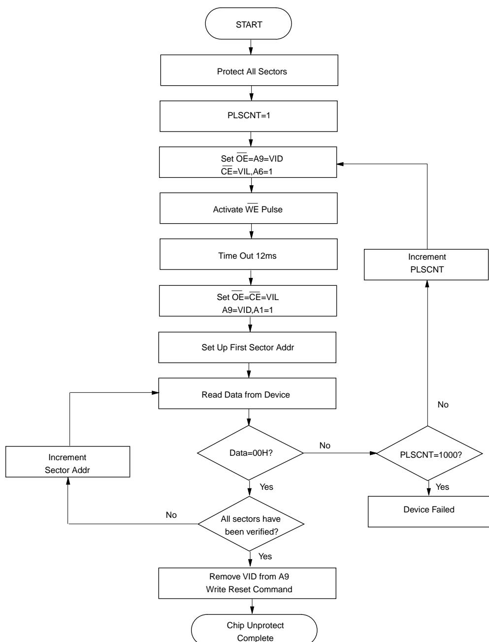
\* It is recommended before unprotect the whole chip, all sectors should be protected in advance.
