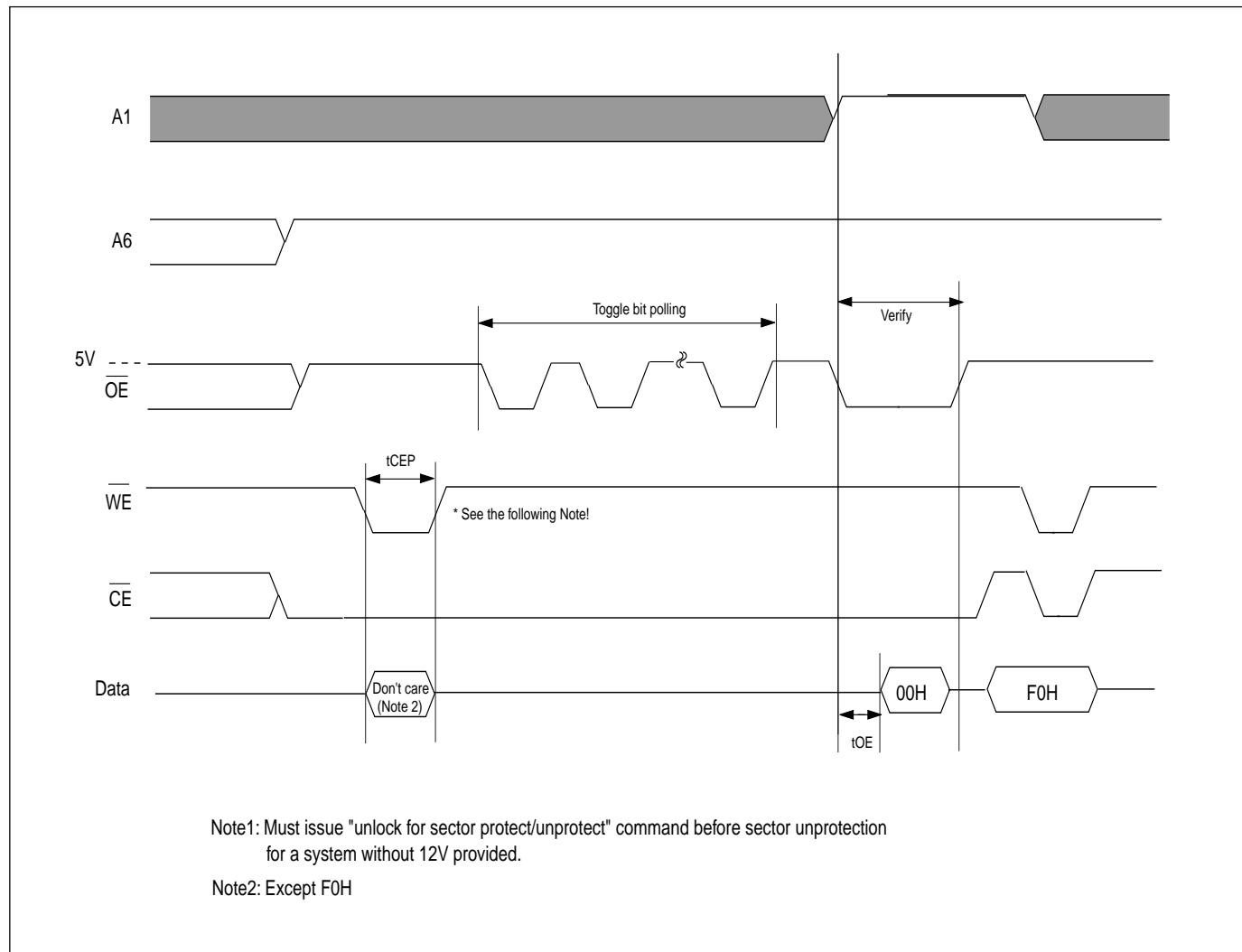
**SECTOR PROTECTION ALGORITHM FOR SYSTEM WITHOUT 12V**
