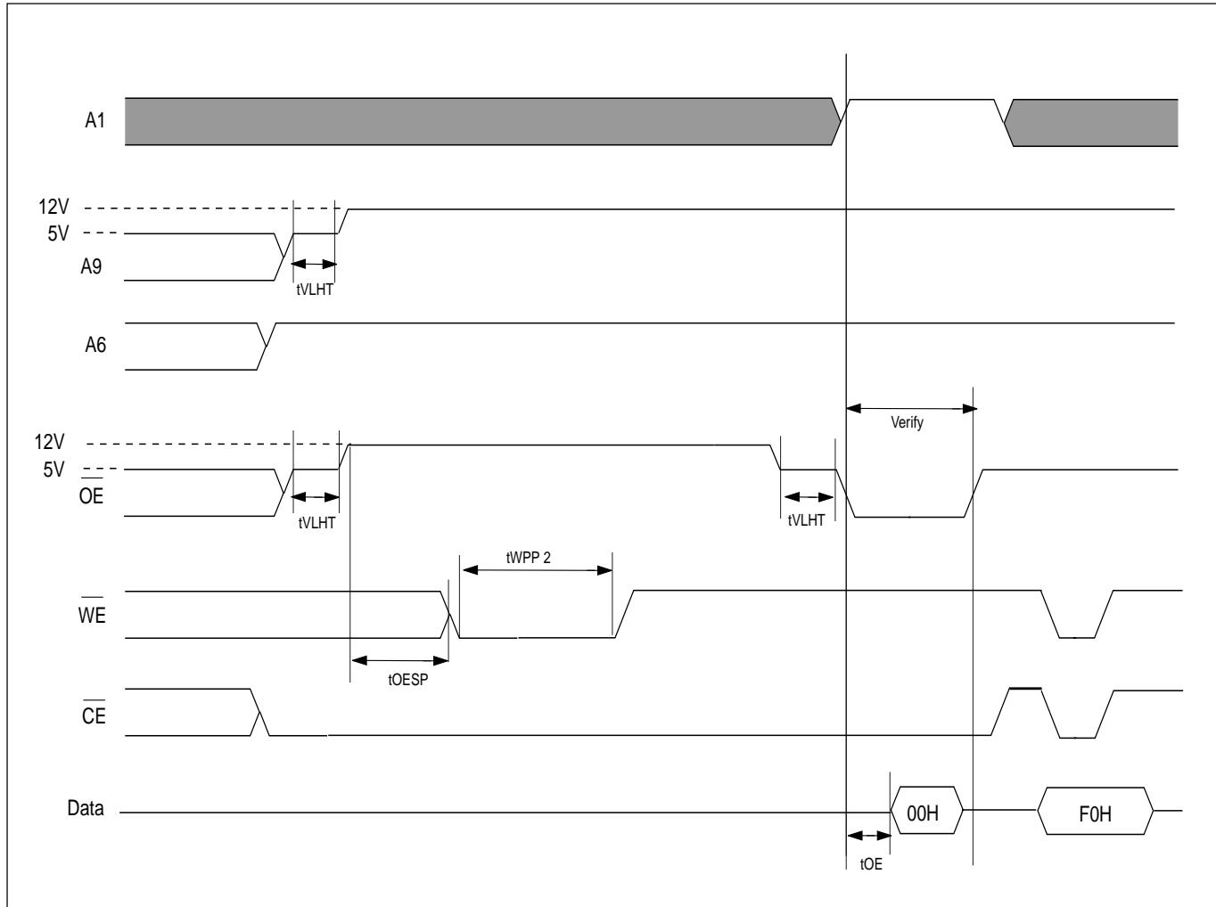
**SECTOR PROTECTION ALGORITHM FOR SYSTEM WITH 12V**
