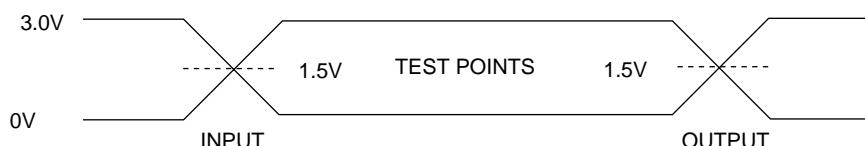
AC TESTING: Inputs are driven at 3.0V for a logic "1" and 0V for a logic "0".
