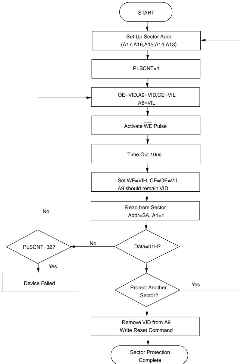
**CHIP UNPROTECTION ALGORITHM FOR SYSTEM WITH 12V**
