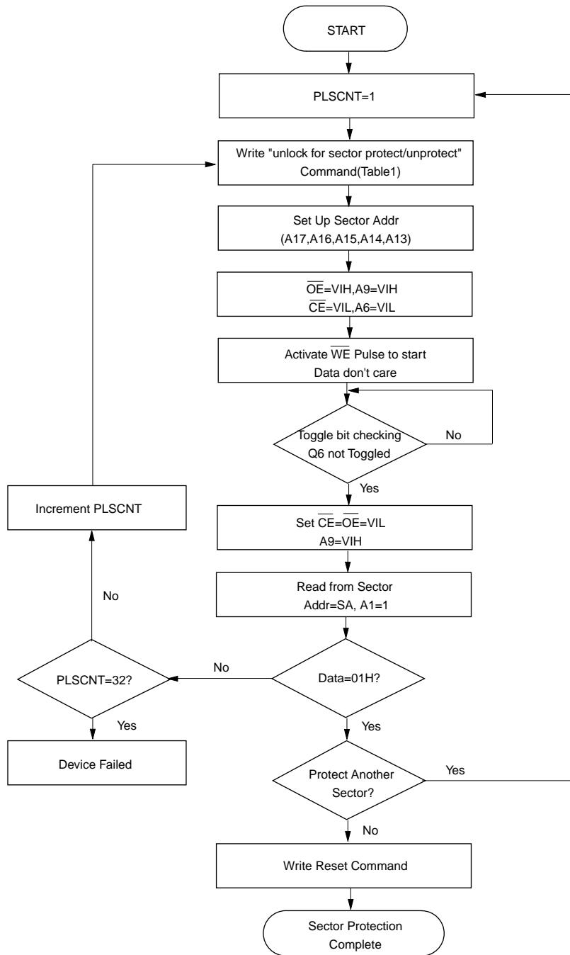
**CHIP UNPROTECTION ALGORITHM FOR SYSTEM WITHOUT 12V**
