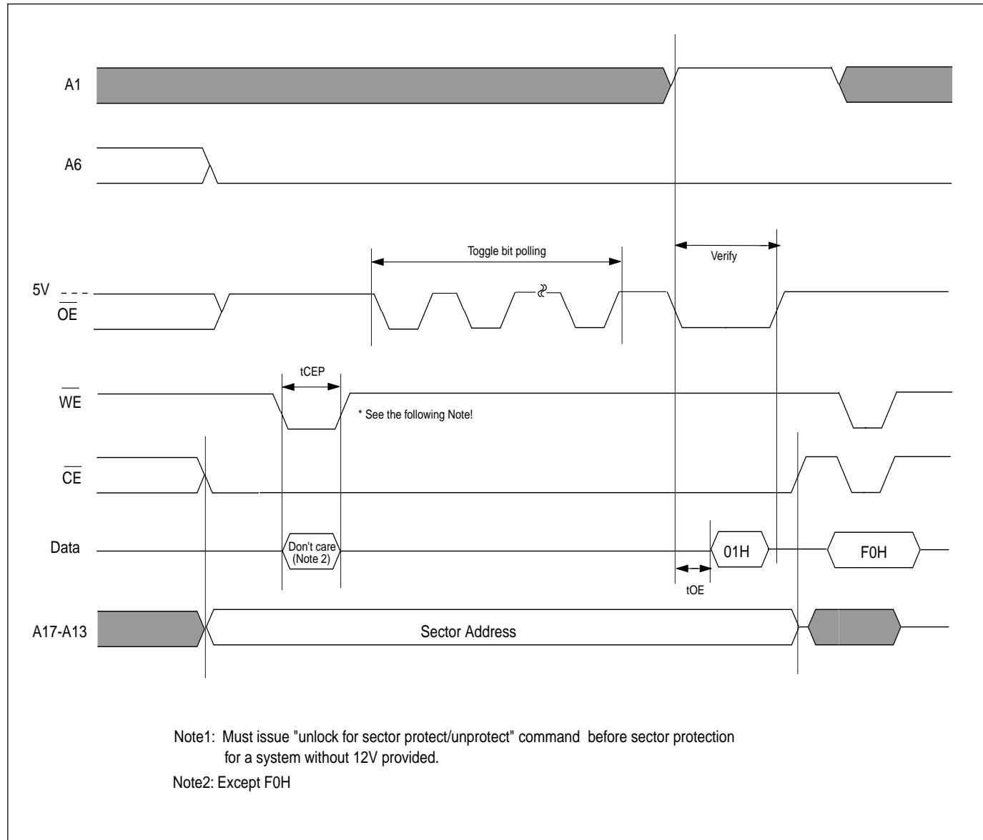
**TIMING WAVEFORM FOR CHIP UNPROTECTION FOR SYSTEM WITHOUT 12V**
