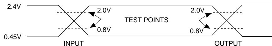
AC TESTING: Inputs are driven at 2.4V for a logic "1" and 0.45V for a logic "0".
