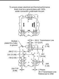
Dimensions are in Inches [Millimeters] 3A425 Rev A Mounting Footprint
