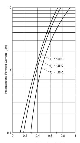
$\label{eq:Forward Voltage Drop-V} Forward\ Voltage\ Drop\ -V_{_{FM}}(V)$  Fig. 1 - Maximum Forward\ Voltage\ Drop\ Characteristics
