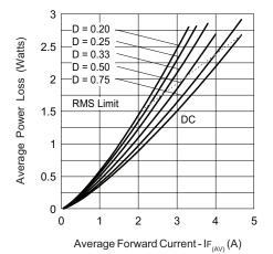
Fig. 5 - Forward Power Loss Characteristics
