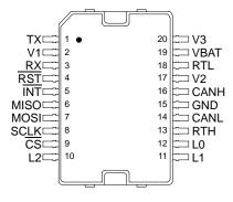
Figure 3. 33389 Pin Connections
