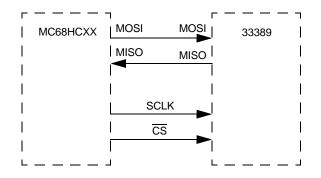
Figure 16. SPI Interface with Microcontroller
