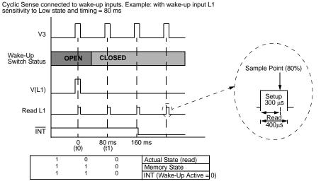
Figure 11. Cyclic Sense Timing
