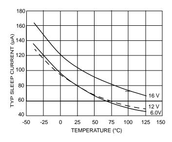
Figure 15. Current vs Temp and Batt Voltage
