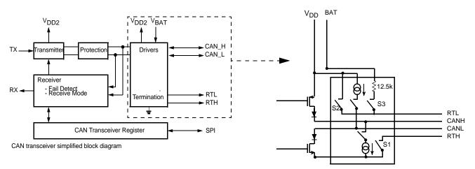
Figure 5. CAN Simplified Block Diagram
