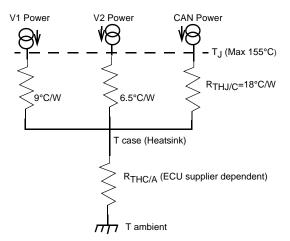
Figure 6. HSOP-20 Simplified Thermal Model
