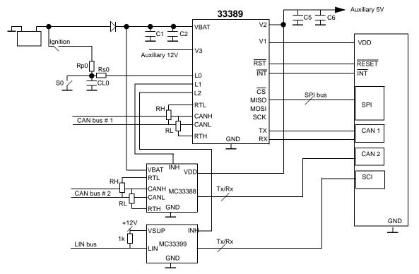
(Wake-up input linked to peripheral circuits: (ex: low speed CAN or LIN transceivers).
