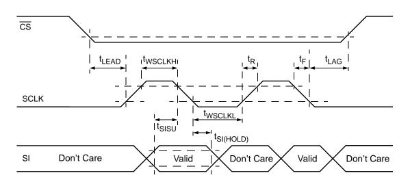
Figure 4. Input Timing Switch Characteristics
