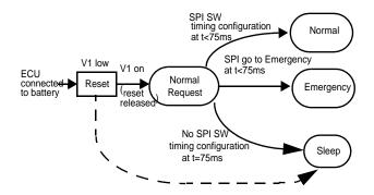
Figure 8. Typical Behavior at Power-On
