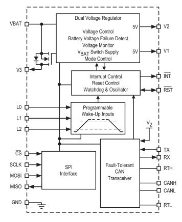
Figure 2. 33389 Simplified Internal Block Diagram
