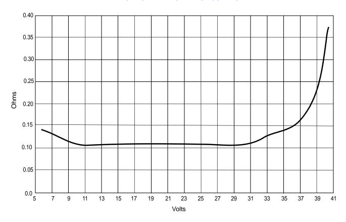
Figure 18. Typical High-Side R<sub>DS(ON)</sub> Versus V+
