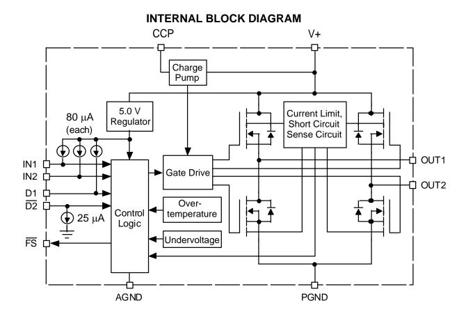
Figure 2. 33886 Simplified Internal Block Diagram
