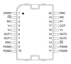
Figure 3. 33886 Pin Connections
