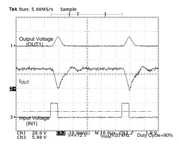
Figure 17. Output Voltage and Current vs. Input Voltage at V+ = 12 V, PMW Frequency of 20 kHz, and Duty Cycle of 90% for a Purely Resistive Load
