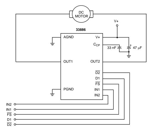
Figure 23. 33886 Typical Application Schematic
