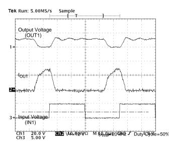
Figure 16. Output Voltage and Current vs. Input Voltage at V+ = 12 V, PMW Frequency of 20 kHz, and Duty Cycle of 50% for a Purely Resistive Load
