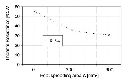
Figure 26. Device on Thermal Test Board  $R_{\theta JA}$
