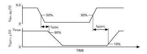
Figure 4. Output Delay Time
