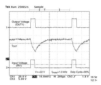
Figure 13. Output Voltage and Current vs. Input Voltage at V+ = 22 V, PMW Frequency of 1.0 kHz, and Duty Cycle of 90%
