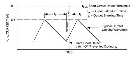
Figure 9. Active Current Limiting Detail
