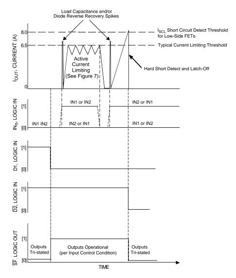
Figure 8. Active Current Limiting Versus Time
