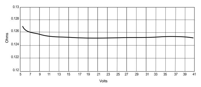
Figure 19. Typical Low-Side  $R_{DS(ON)}$  Versus V+
