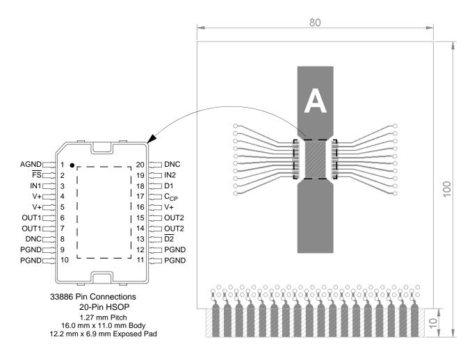
Figure 25. Thermal Test Board
