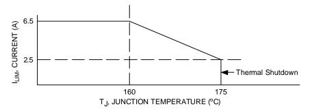
Figure 7. Active Current Limiting Versus Temperature (Typical)
