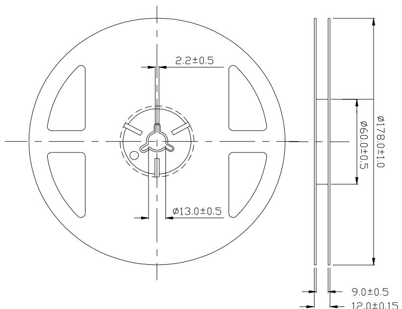
**Note:** The tolerances unless mentioned is  $\pm 0.1\text{mm}$ , Unit = mm
