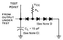
LOAD FOR OUTPUT UNDER TEST
