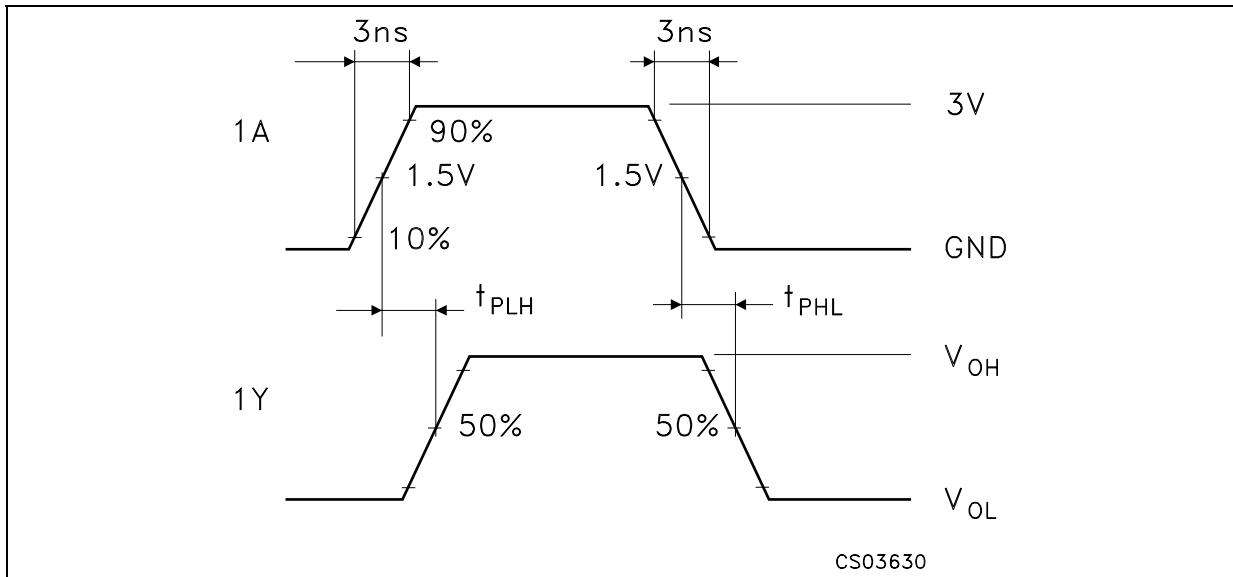
**WAVEFORM 2: OUTPUT ENABLE AND DISABLE TIME (f=1MHz; 50% duty cycle)**
