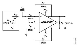
Figure 50. Calculating Single-Ended Input Impedance RIN
