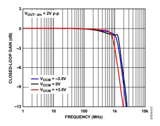
Figure 17. Large Signal Frequency Response at Various V<sub>OCM</sub> Levels
