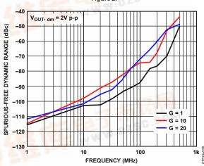
Figure 3. Spurious-Free Dynamic Range vs. Frequency at Various Gains
