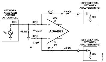
Figure 44. Test Circuit for Output Balance, CMRR
