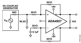
Figure 43. Equivalent Basic Test Circuit, G = 1
