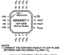
Figure 5. ADA4927-1 Pin Configuration
