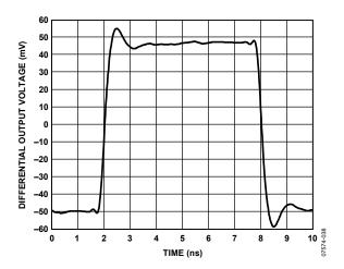
Figure 38. Vocm Small Signal Pulse Response
