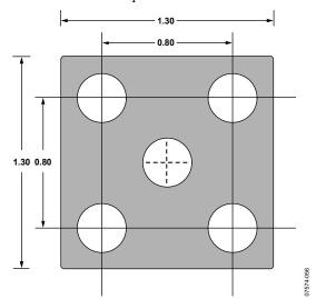
Figure 56. Recommended PCB Thermal Attach Pad Dimensions (Millimeters)
