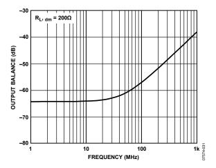
Figure 31. Output Balance vs. Frequency
