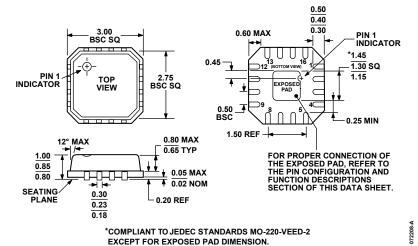
Figure 59. 16-Lead Lead Frame Chip Scale Package [LFCSP\_VQ] 3 mm × 3 mm Body, Very Thin Quad (CP-16-2) Dimensions shown in millimeters
