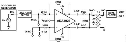
Figure 45. Test Circuit for Distortion Measurements
