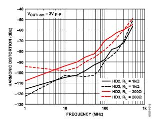
Figure 19. Harmonic Distortion vs. Frequency at Various Loads
