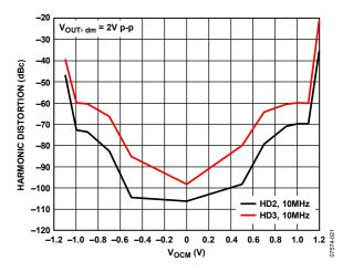
Figure 21. Harmonic Distortion vs. V<sub>OCM</sub> at 10 MHz, ±2.5 V Supplies
