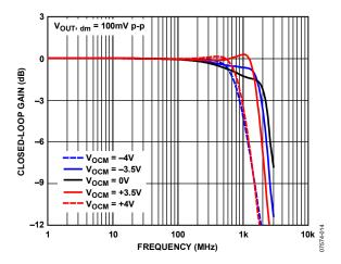
Figure 14. Small Signal Frequency Response at Various V<sub>OCM</sub> Levels
