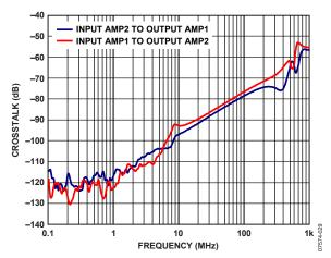
Figure 29. Crosstalk vs. Frequency for ADA4927-2
