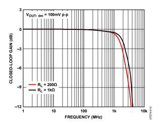
Figure 13. Small Signal Frequency Response for Various Loads
