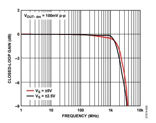
Figure 8. Small Signal Frequency Response for Various Supplies
