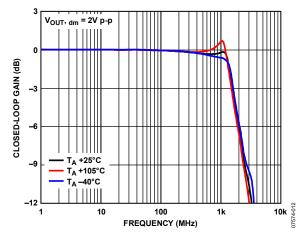
Figure 12. Large Signal Frequency Response for Various Temperatures
