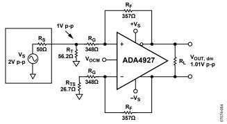
Figure 54. Terminated Single-Ended-to-Differential System with G = 1
