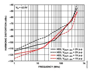
Figure 25. Harmonic Distortion vs. Frequency at Various V<sub>OUT, dm</sub>
