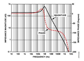
Figure 34. Open-Loop Transimpedance Magnitude and Phase vs. Frequency
