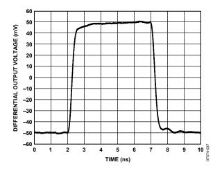
Figure 37. Small Signal Pulse Response
