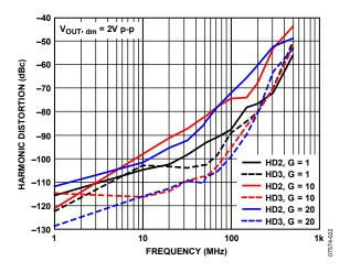
Figure 22. Harmonic Distortion vs. Frequency at Various Gains
