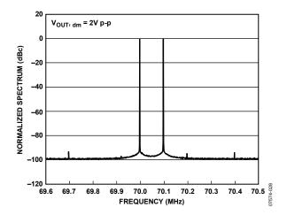
Figure 28. 70 MHz Intermodulation Distortion
