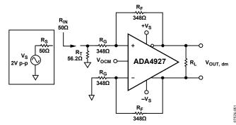
Figure 51. Adding Termination Resistor R<sub>T</sub>
