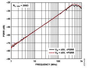
Figure 30. PSRR vs. Frequency
