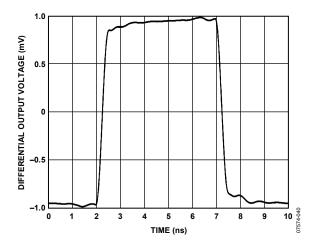
Figure 40. Large Signal Pulse Response
