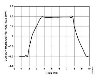
Figure 41. Vocm Large Signal Pulse Response
