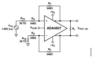
Figure 53. Thevenin Equivalent and Matched Gain Resistors
