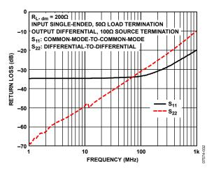
Figure 32. Return Loss (S<sub>11</sub>, S<sub>12</sub>) vs. Frequency
