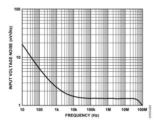
Figure 33. Voltage Noise Spectral Density, Referred to Input
