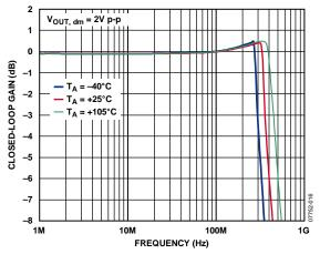
Figure 16. Large Signal Frequency Response for Various Temperatures
