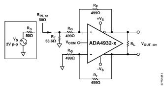
Figure 60. Adding Termination Resistor,  $R_T$
