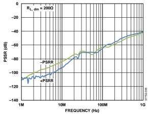
Figure 36. PSRR vs. Frequency
