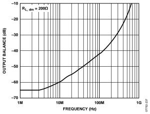
Figure 37. Output Balance vs. Frequency
