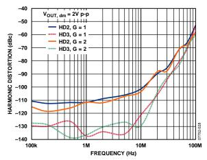
Figure 28. Harmonic Distortion vs. Frequency at Various Gains
