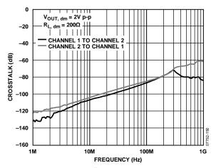
Figure 50. Crosstalk vs. Frequency, ADA4932-2
