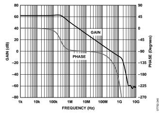
Figure 40. Open-Loop Gain and Phase vs. Frequency
