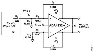
Figure 63. Terminated Single-Ended-to-Differential System with G = 2
