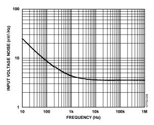
Figure 39. Voltage Noise Spectral Density, Referred to Input
