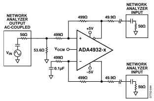
Figure 53. Test Circuit for Output Balance, CMRR
