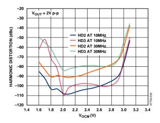
Figure 30. Harmonic Distortion vs.  $V_{\rm OCM}$  at Various Frequencies, +5 V Supply
