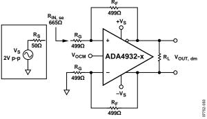
Figure 59. Calculating Single-Ended Input Impedance,  $R_{IN}$
