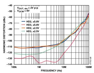
Figure 26. Harmonic Distortion vs. Frequency at Various Supplies
