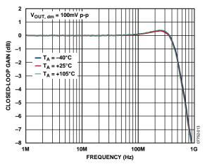
Figure 13. Small Signal Frequency Response for Various Temperatures
