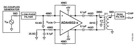
Figure 54. Test Circuit for Distortion Measurements
