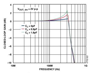
Figure 22. Large Signal Frequency Response at Various Capacitive Loads
