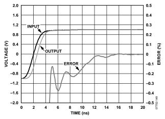
Figure 49. Settling Time
