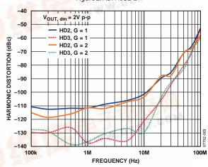
Figure 3. Harmonic Distortion vs. Frequency at Various Gains
