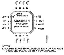
Figure 5. ADA4932-1 Pin Configuration
