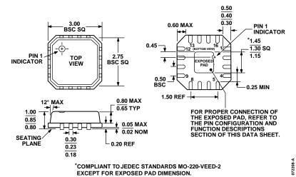
Figure 68. 16-Lead Lead Frame Chip Scale Package [LFCSP\_VQ] 3 mm × 3 mm Body, Very Thin Quad (CP-16-2) Dimensions shown in millimeters
