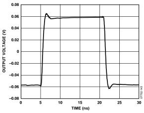
Figure 43. Small Signal Pulse Response
