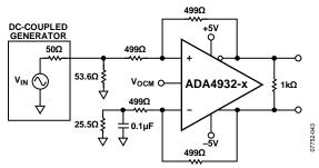
Figure 52. Equivalent Basic Test Circuit, G = 1
