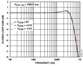
Figure 15. Small Signal Frequency Response for Various  $V_{\text{OCM}}$  Levels
