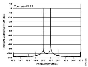
Figure 35. 30 MHz Intermodulation Distortion
