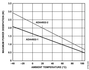
Figure 4. Maximum Power Dissipation vs. Ambient Temperature for a 4-Laver Board
