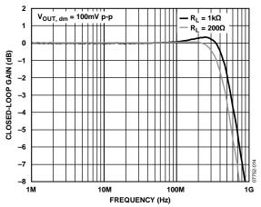
Figure 14. Small Signal Frequency Response at Various Loads
