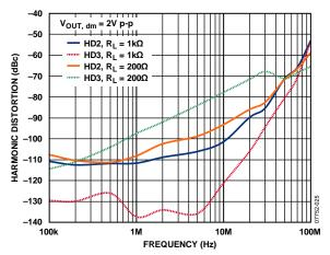
Figure 25. Harmonic Distortion vs. Frequency at Various Loads
