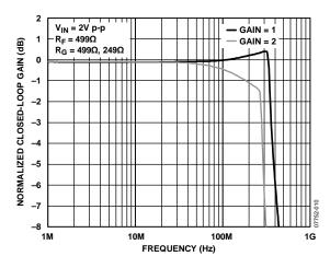
Figure 10. Large Signal Frequency Response for Various Gains
