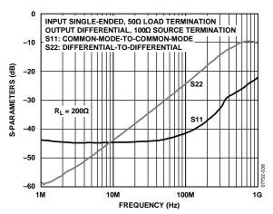
Figure 38. Return Loss  $(S_{11}, S_{22})$  vs. Frequency
