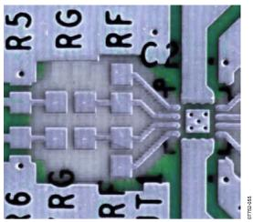
Figure 64. Ground and Power Plane Voiding in Vicinity of  $R_F$  and  $R_G$
