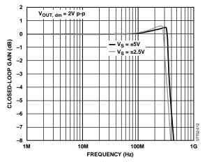
Figure 12. Large Signal Frequency Response for Various Supplies
