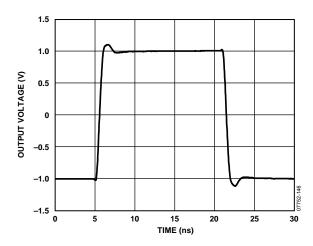
Figure 46. Large Signal Pulse Response
