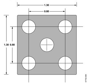
Figure 65. Recommended PCB Thermal Attach Pad Dimensions (Millimeters)
