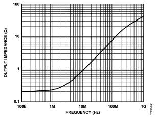
Figure 41. Closed-Loop Output Impedance Magnitude vs. Frequency, G = 1
