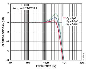
Figure 19. Small Signal Frequency Response at Various Capacitive Loads
