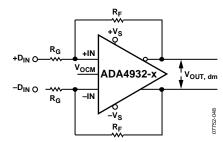
Figure 57. ADA4932-x Configured for Balanced (Differential) Inputs
