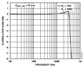
Figure 17. Large Signal Frequency Response at Various Loads
