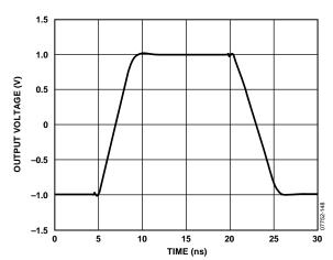
Figure 48.  $V_{OCM}$  Large Signal Pulse Response
