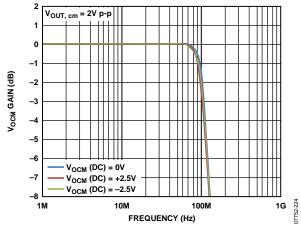
Figure 24. V<sub>OCM</sub> Large Signal Frequency Response at Various DC Levels
