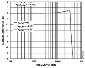
Figure 18. Large Signal Frequency Response for Various  $V_{\text{OCM}}$  Levels
