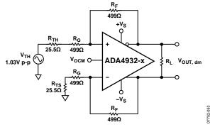
Figure 62. Thevenin Equivalent and Matched Gain Resistors
