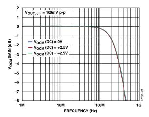
Figure 21.  $V_{\rm OCM}$  Small Signal Frequency Response at Various DC Levels
