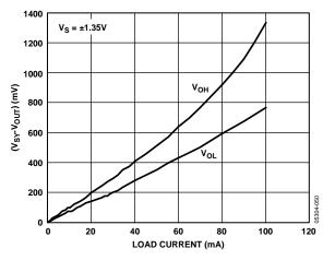
Figure 37. AD8655 Output Voltage to Supply Rail vs. Load Current
