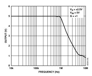
Figure 26. Maximum Output Swing vs. Frequency
