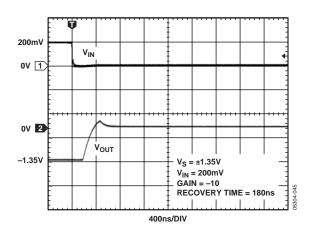
Figure 45. Negative Overload Recovery Time
