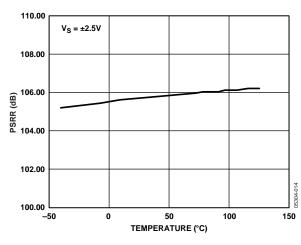
Figure 19. Large Signal PSSR vs. Temperature
