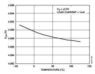
Figure 14. Output Voltage Swing High vs. Temperature
