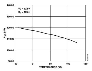
Figure 24. Large Signal Open-Loop Gain vs. Temperature
