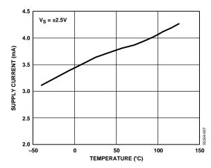
Figure 11. Supply Current vs. Temperature
