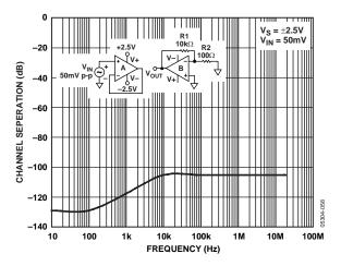
Figure 55. Channel Separation vs. Frequency
