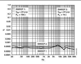
Figure 60. THD + Noise vs. Frequency
