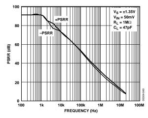
Figure 49. Small Signal PSSR vs. Frequency
