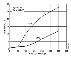
Figure 29. Small Signal Overshoot vs. Load Capacitance
