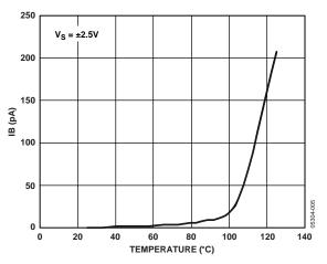
Figure 9. Input Bias Current vs. Temperature
