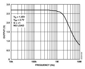
Figure 53. Maximum Output Swing vs. Frequency
