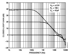
Figure 25. Closed-Loop Gain vs. Frequency
