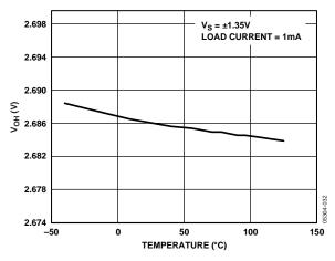
Figure 39. Output Voltage Swing High vs. Temperature
