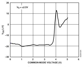
Figure 8. Input Offset Voltage vs. Common-Mode Voltage
