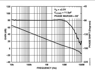
Figure 23. Open-Loop Gain and Phase vs. Frequency
