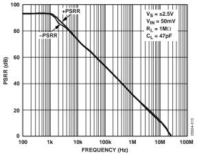
Figure 18. Small Signal PSSR vs. Frequency
