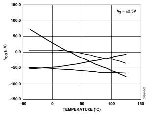
Figure 6. Input Offset Voltage vs. Temperature
