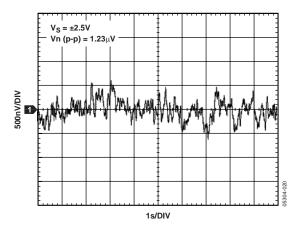
Figure 21. Low Frequency Noise (0.1 Hz to 10 Hz).
