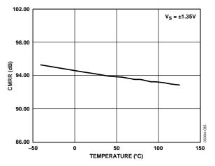
Figure 48. Large Signal CMRR vs. Temperature
