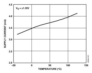
Figure 36. Supply Current vs. Temperature
