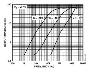
Figure 32. Output Impedance vs. Frequency
