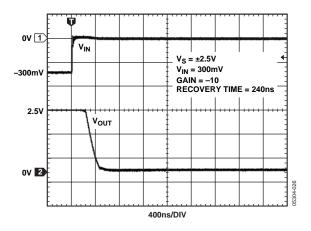
Figure 31. Positive Overload Recovery Time
