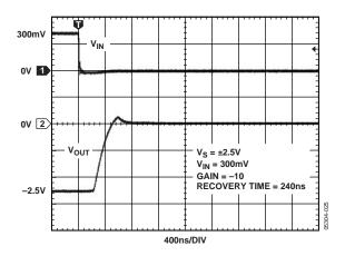
Figure 30. Negative Overload Recovery Time
