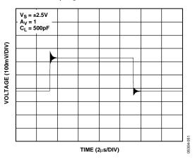
Figure 56. Driving Heavy Capacitive Loads Without Compensation
