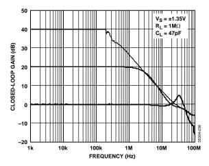
Figure 52. Closed-Loop Gain vs. Frequency
