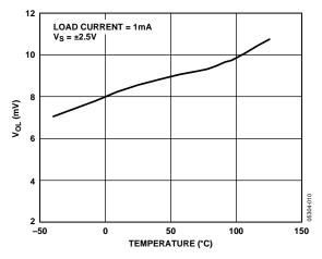
Figure 15. Output Voltage Swing Low vs. Temperature
