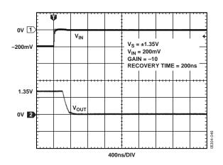
Figure 46. Positive Overload Recovery Time
