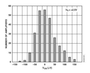
Figure 5. Input Offset Voltage Distribution
