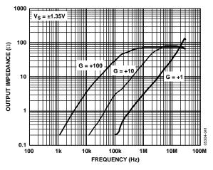
Figure 54. Output Impedance vs. Frequency
