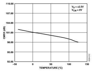
Figure 17. Large Signal CMRR vs. Temperature
