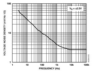
Figure 20. Voltage Noise Density vs. Frequency
