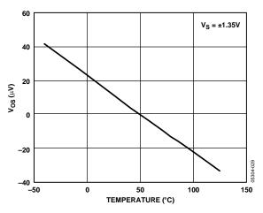
Figure 34. Input Offset Voltage vs. Temperature
