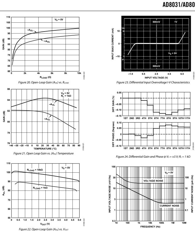
Figure 25. Input Voltage Noise vs. Frequency
