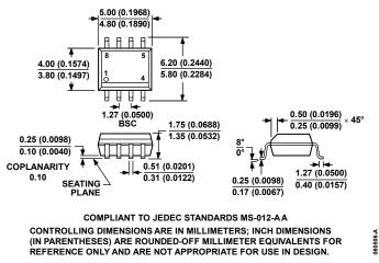
Figure 55. 8-Lead Standard Small Outline Package [SOIC\_N] Narrow Body (R-8) Dimensions shown in millimeters and (inches)
