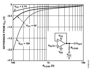
Figure 15. +Output Saturation Voltage vs. R<sub>LOAD</sub> @ +25°C
