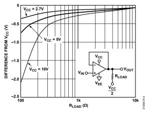
Figure 14. +Output Saturation Voltage vs. R<sub>LOAD</sub> @ +85°C
