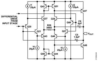
Figure 44. Output Stage Simplified Schematic
