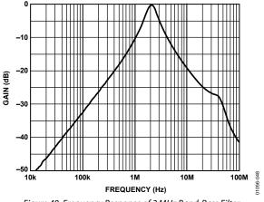
Figure 48. Frequency Response of 2 MHz Band-Pass Filter
