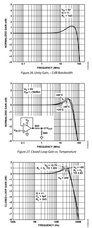
Figure 28. Closed-Loop Gain vs. Supply Voltage
