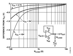
Figure 16. +Output Saturation Voltage vs. RLOAD @ -40°C
