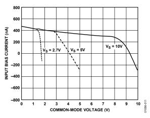
Figure 11. Input Bias Current vs. Common-Mode Voltage
