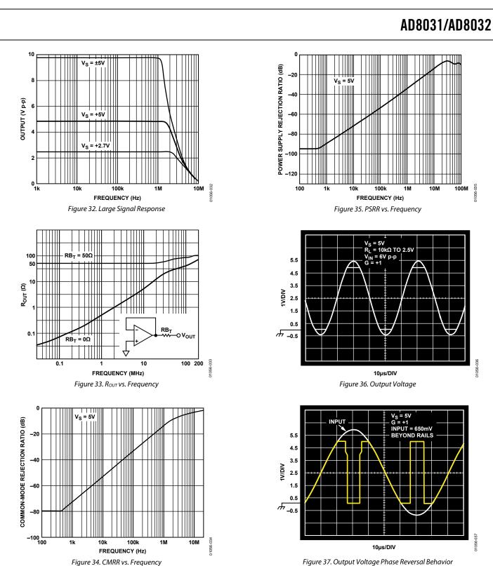
Figure 37. Output Voltage Phase Reversal Behavior
