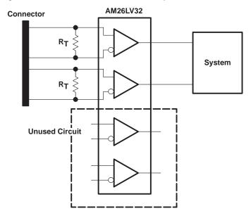
Figure 9. Typical Application with Unused Receivers
