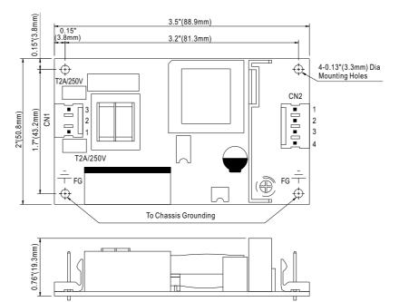
AC Input Connector (CN1): Molex 41791-03 or equivalent
