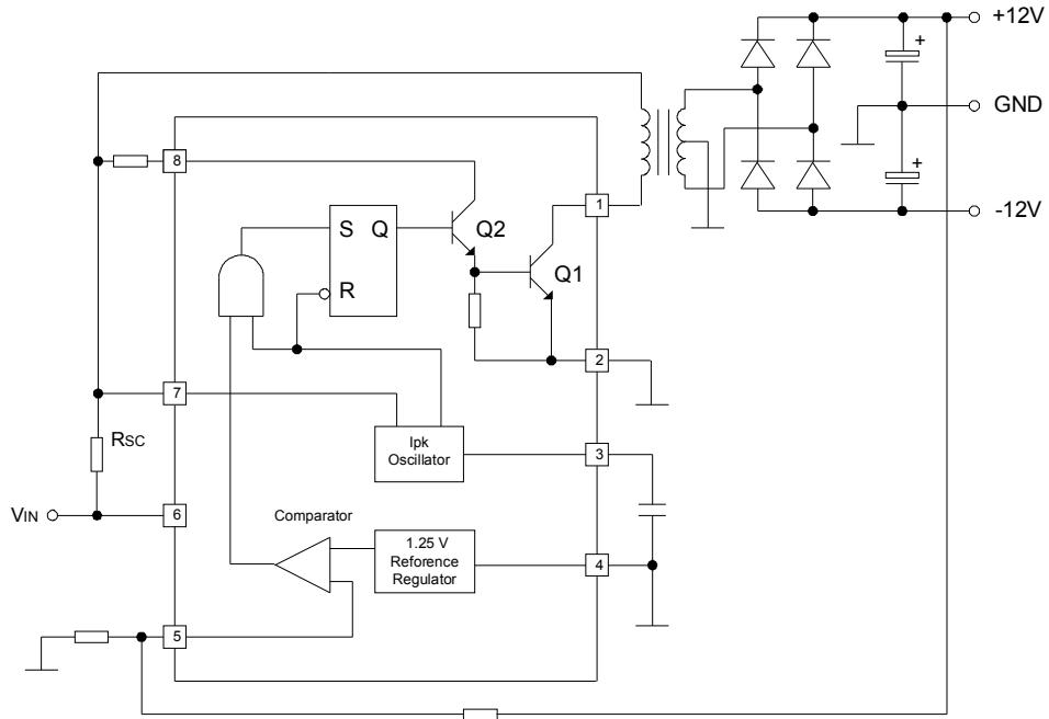
Higher Output Power, Higher Input Voltage
