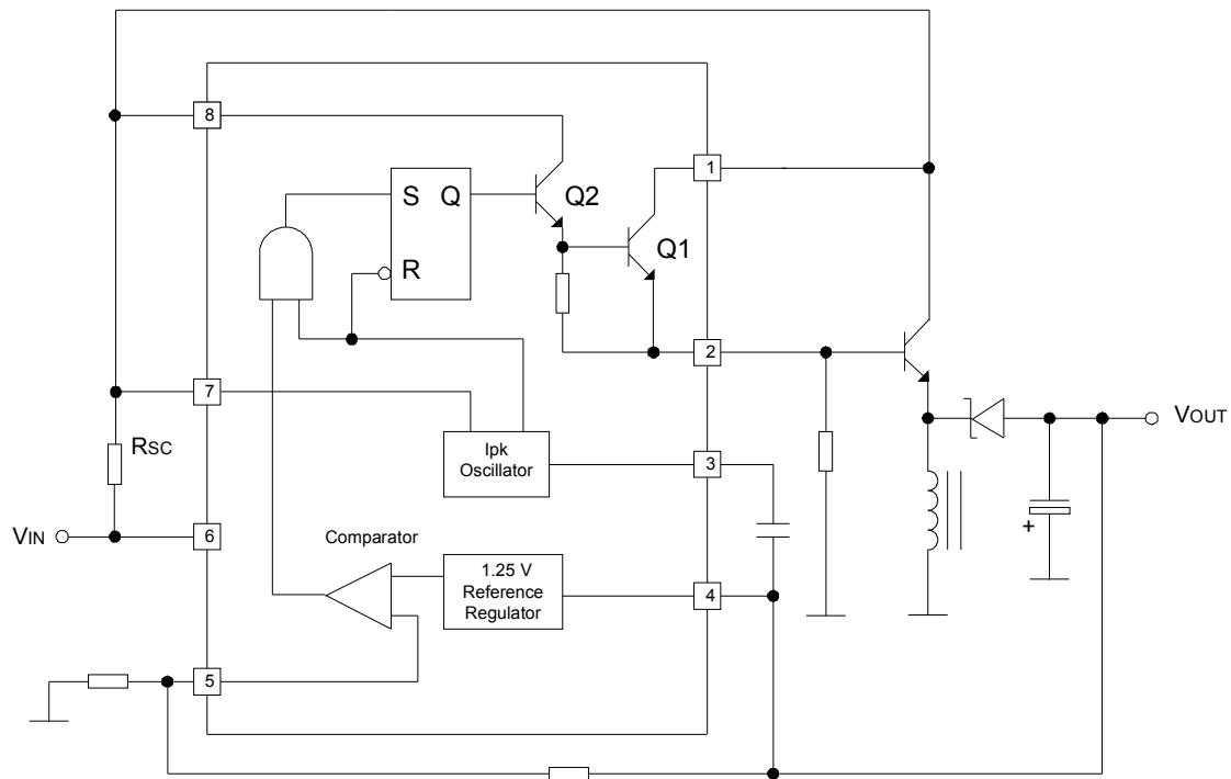
Voltage Inverting With External PNP Saturated Switch
