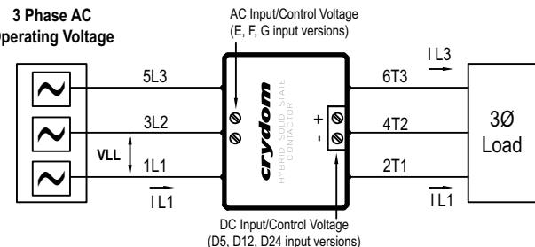
DO NOT apply any AC voltage to contactor coil connections, for DC versions only.
