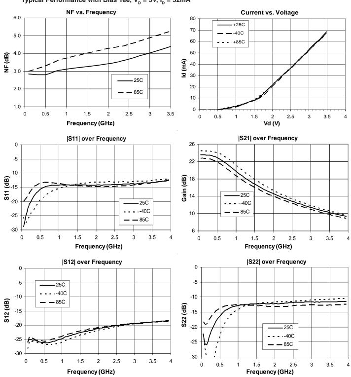
Typical Performance with Bias Tee,  $V_{D} = 3V$ ,  $I_{D} = 52mA$
