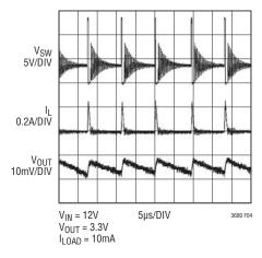
Figure 4. Burst Mode Operation
