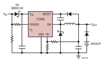
Figure 8. Diode D4 Prevents a Shorted Input from Discharging a Backup Battery Tied to the Output. It Also Protects the Circuit from a Reversed Input. The LT3680 Runs Only When the Input is Present
