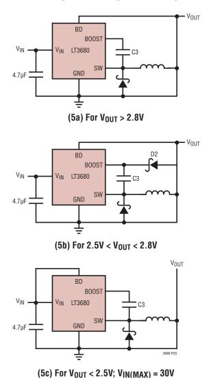
Figure 5. Three Circuits For Generating The Boost Voltage
