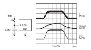
Figure 7. To Soft-Start the LT3680, Add a Resisitor and Capacitor to the RUN/SS Pin
