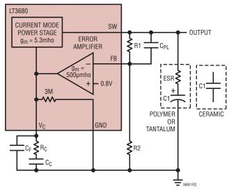
Figure 2. Model for Loop Response
