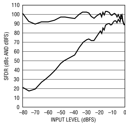
SFDR vs 30.2MHz Input Level, PGA = 0
