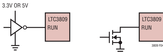
Figure 4. RUN Pin Interfacing
