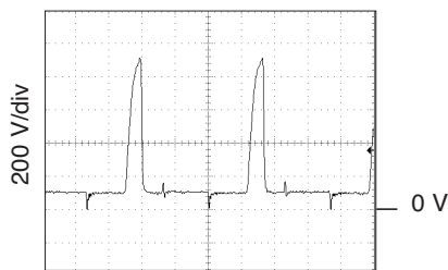
500 ns/div Representative of all models MOR2812D Sync Out FIGURE 29
