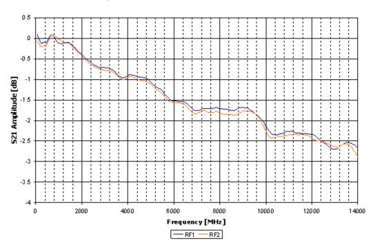
DDMZ S21 Electro-optic Phase Response Characteristics
