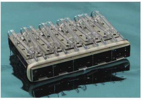
Lightpipe cover mounted on 1-by-5 SFP cage
