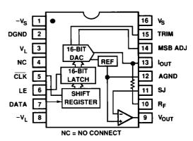
The serial interface consists of bit clock, data, and latch enable inputs. The twos-complement data word is clocked MSB first on falling clock edges into the serial-to-parallel converter, consistent with the serial protocols of popular DSP processors. The input clock can support data transfers up to 12.5 MHz. The falling edge of latch enable updates the internal DAC input register at the sample rate with the sixteen bits most recently clocked into the serial input register.
