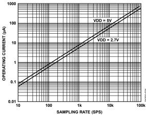
Figure 24. Operating Current vs. Sampling Rate
