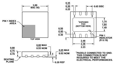
Figure 27. 8-Terminal Quad Flat No Lead Package (QFN) [LFCSP\_WD] 3 mm × 3 mm Body, Very Very Thin, Dual Lead (CP-8-3) Dimensions Shown in millimeters 022808-B
