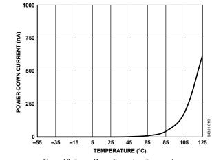
Figure 18. Power-Down Current vs. Temperature
