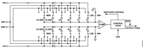
Figure 20. ADC Simplified Schematic
