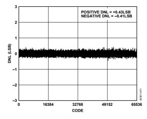
Figure 10. Differential Nonlinearity vs. Code
