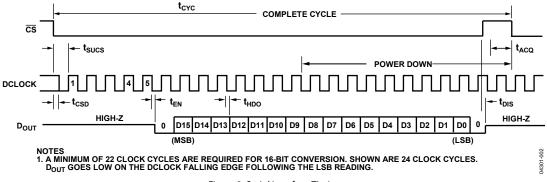
Figure 2. Serial Interface Timing
