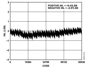
Figure 7. Integral Nonlinearity vs. Code
