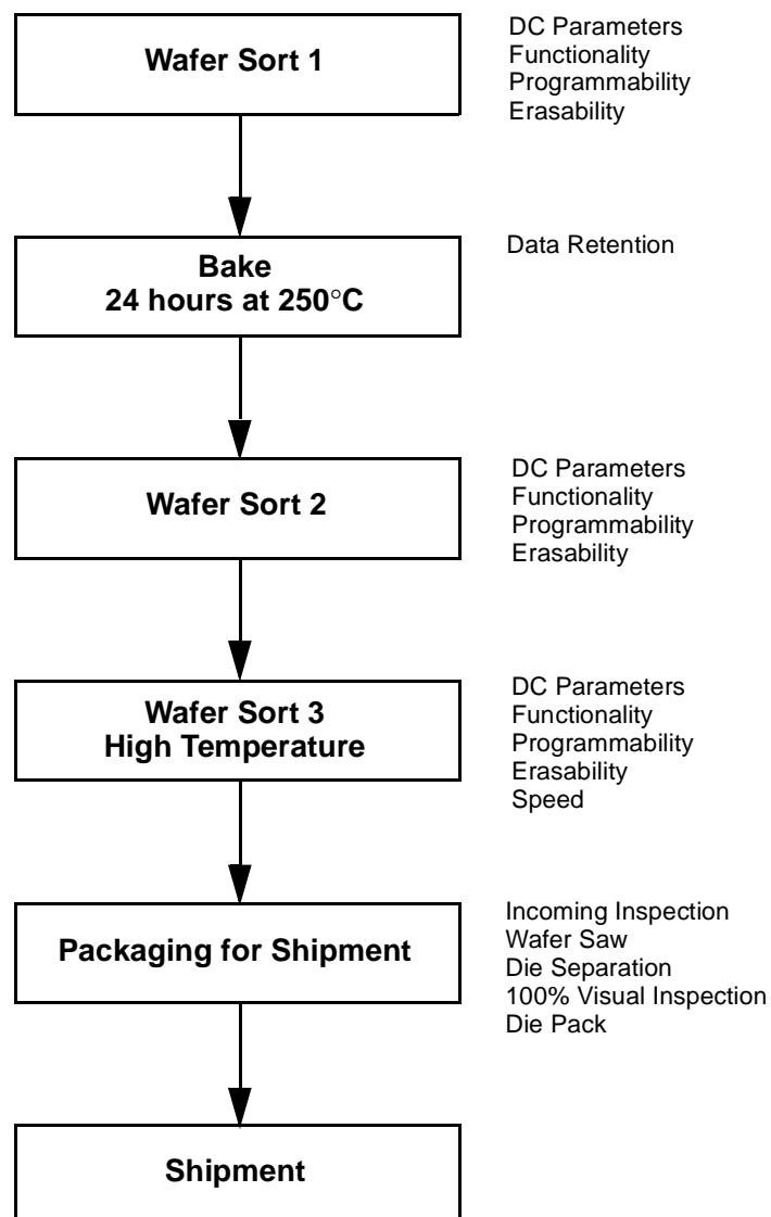
Figure 1. AMD KGD Product Test Flow
