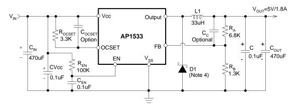
$$V_{OUT} = V_{FB} x (1+R_A/R_B)$$
