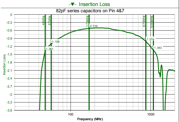
Figure 1 The Balun with external capacitors on both low impedance ports (nominal/test configuration). The two capacitors improve the insertion loss and return loss in the 40-200MHz range over that of the basic balun.
