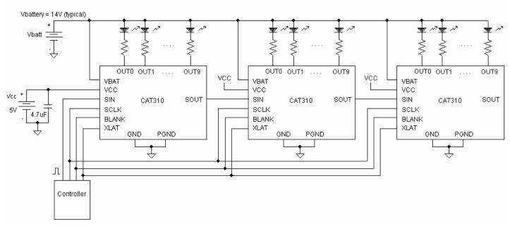
Figure 1. Daisy Chain Application Diagram
