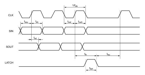
Figure 1. Serial Input Timing Diagram
