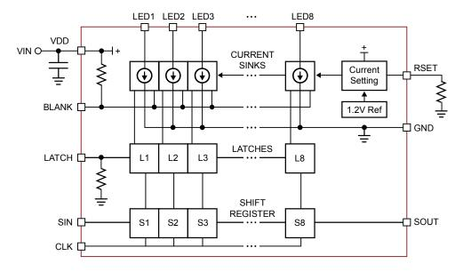
Figure 2. CAT4008 Functional Block Diagram
