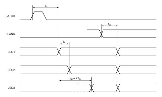
Figure 2. LED Output Timing Diagram
