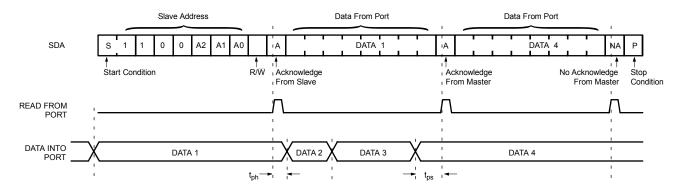
Figure 8. Read Input Port Register Timing Diagram
