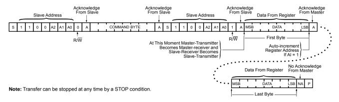
Figure 7. Read from Register Timing Diagram
