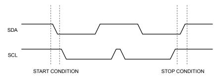
Figure 2. Start/Stop Timing
