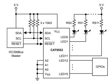
Notes: LED0 to LED11 are shown being used as LED drivers LED12 to LED15 are used as standard GPIOs
