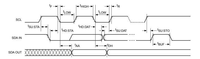
Figure 1. 2-Wire Serial Interface Timing
