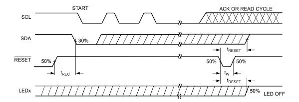
Figure 9. RESET Timing Diagram
