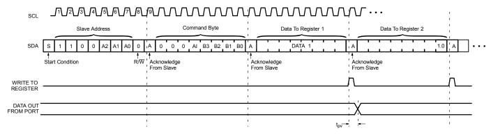
Figure 6. Write to Register Timing Diagram
