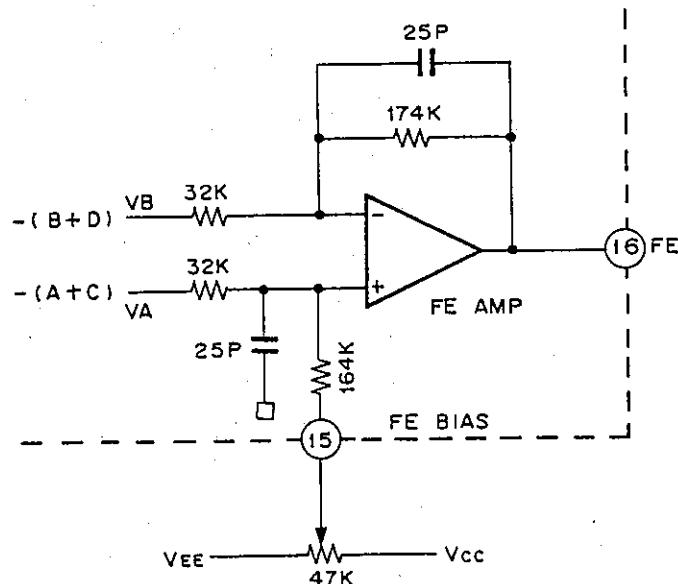
$$\begin{aligned} \text{FE output voltage (low frequency) turns to } V_{\text{FE}} &= 5.4 \times (V_A - V_B) \\ &= (i_{\text{PD2}} - i_{\text{PD1}}) \times 315\text{k}\Omega. \end{aligned}$$
