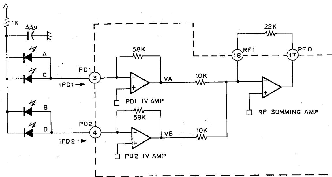
$$\begin{aligned} \text{RFO output voltage low frequency turns to } V_{\text{RFO}} &= 2.2 \times (V_A + V_B) \\ &= 127.6\text{k}\Omega \times (i_{\text{PD1}} + i_{\text{PD2}}). \end{aligned}$$
