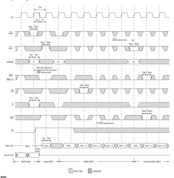
18. Full width Write can be initiated by either  $\overline{GW}$  LOW; or by  $\overline{GW}$  HIGH,  $\overline{BWE}$  LOW and  $\overline{BW}_{[A:D]}$  LOW.
