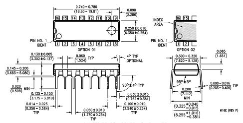
16-Lead Molded Dual-In-Line Package (N) Order Number DM74LS192N NS Package Number N16E
