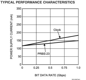
Dynamic power supply current was measured while running a clock or PRBS 2<sup>23</sup>-1 pattern with all 4 channels active. V<sub>CC</sub> = 3.3V, T<sub>A</sub> = +25°C, V<sub>ID</sub> = 0.5V, V<sub>CM</sub> = 1.2V
