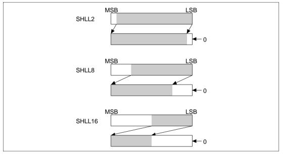
Figure 6.11 Shift Logical Left n Bits
