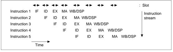
Figure 7.1 Basic Structure of Pipeline Flow
