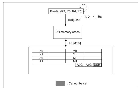
Figure 4.21 Single Data Transfer Flowchart (Longword)
