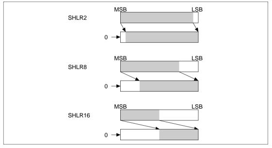
Figure 6.13 Shift Logical Right n Bits
