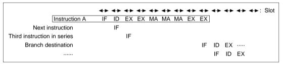
Figure 7.93 TRAP Instruction Pipeline
