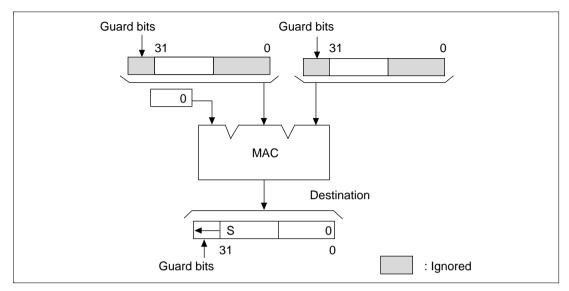
Figure 4.13 shows a flowchart of fixed decimal point multiplication.
