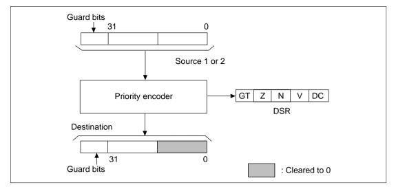
Figure 4.16 MSB Detection Flowchart
