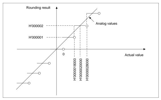
Figure 4.18 Rounding Process Definitions
