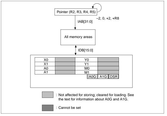
Figure 4.20 Single Data Transfer Flowchart (Word)
