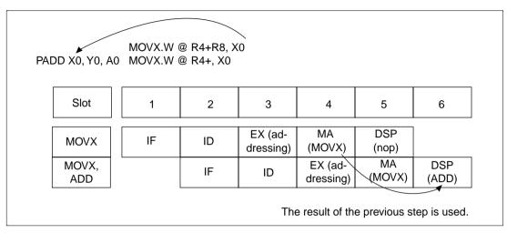
Figure 4.7 Sample Processing Flowchart
