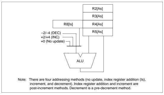
Figure 4.2 Single Data Transfer Addressing
