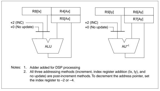
Figure 4.1 X and Y Data Transfer Addressing
