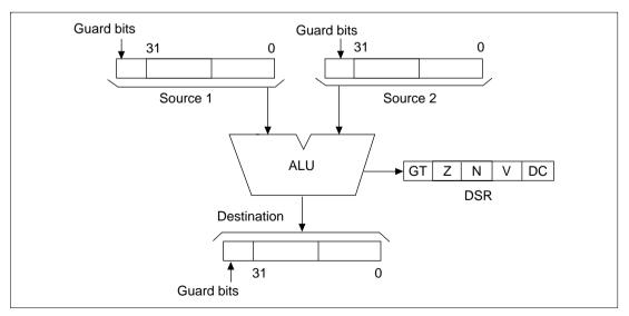
Figure 4.6 ALU Fixed Decimal Point Operation Flowchart
