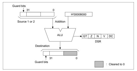
Figure 4.17 Rounding Flowchart
