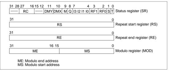
Figure 2.4 Organization of the Control Registers (SH-DSP)
