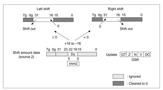
Figure 4.15 shows the logical shift operation flowchart.
