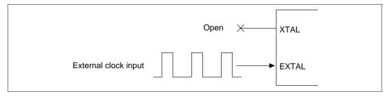
Figure 7.4 External Clock Input Method
