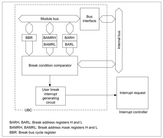
Figure 6.1 Block Diagram of User Break Controller
