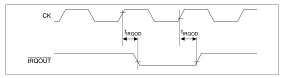
Figure 20.50 Interrupt Signal Output Timing
