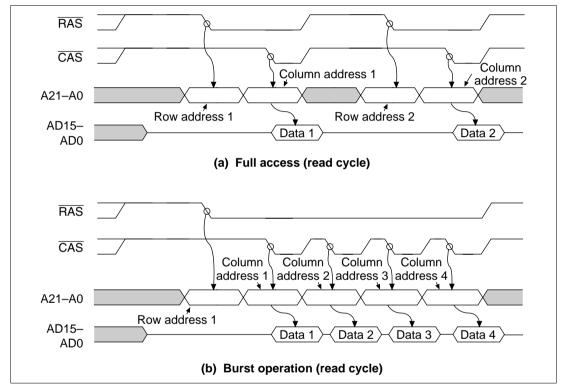
Figure 8.22 Full Access and Burst Operation
