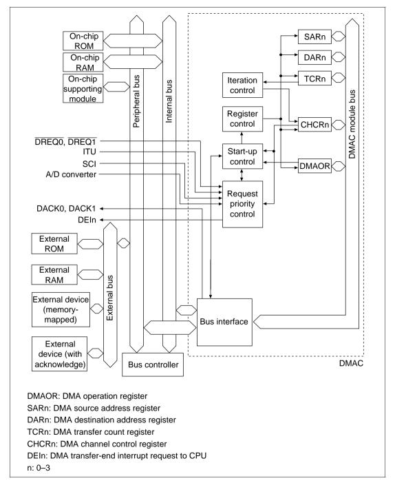
Figure 9.1 Block Diagram of DMAC
