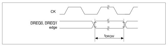
Figure 20.35 DREQ0, DREQ1 Input Timing (2)
