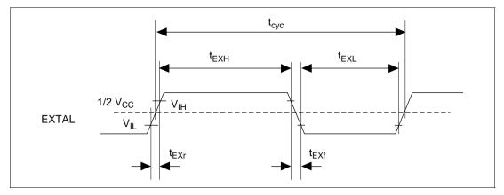
Figure 20.45 EXTAL Input Timing
