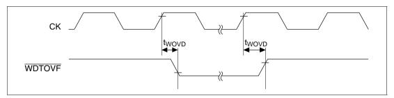
Figure 20.70 Watchdog Timer Output Timing
