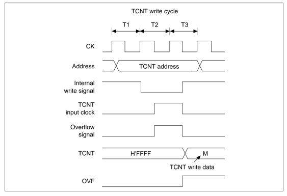
Figure 10.62 Contention between TCNT Write and Overflow
