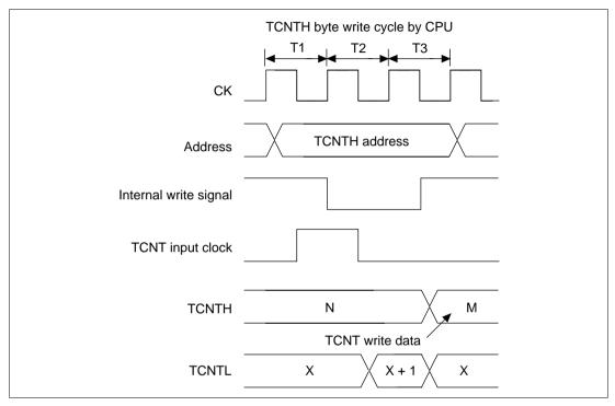
Figure 10.60 Contention between TCNT Byte Write and Increment
