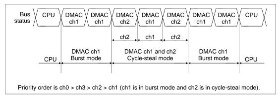
Figure 9.12 Bus Handling when Multiple Channels are Operating
