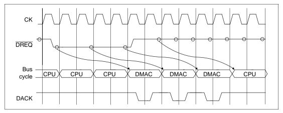
Figure 9.23 DREQ Pin Sampling Timing in Burst Mode (Single Address DREQ Level Detection, DACK Active-Low, 1 Bus Cycle = 2 States)
