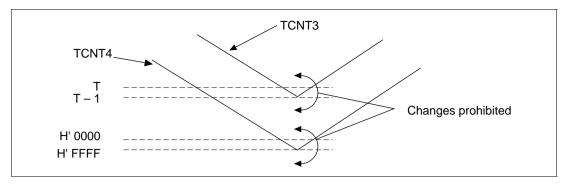
Figure 10.40 Caution on Changing GR Settings with Buffer Operation (2)
