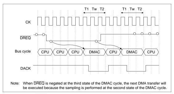
Figure 9.17  $\overline{DREQ}$  Sampling Timing in Cycle-Steal Mode (Output with  $\overline{DREQ}$  Level Detection and DACK Active-Low) (Single Address Mode, Bus Cycle = 2 States + 1 Wait State)
