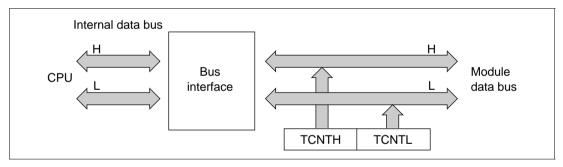
Figure 10.7 TCNT Access (TCNT to CPU (Word))
