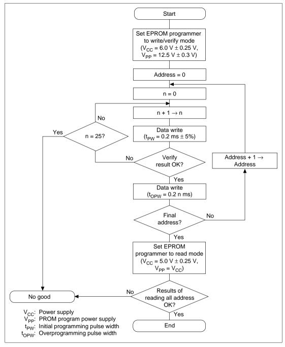
Figure 17.4 Basic Flowchart of High-Speed, High-Reliability Programming
