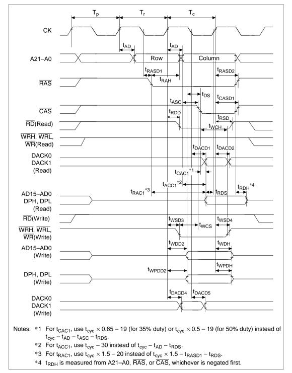
Figure 20.11 DRAM Bus Cycle (Short-Pitch, Normal Mode)
