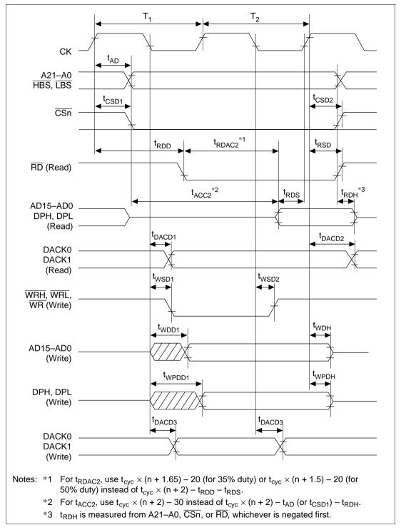
Figure 20.9 Basic Bus Cycle: Two-State Access
