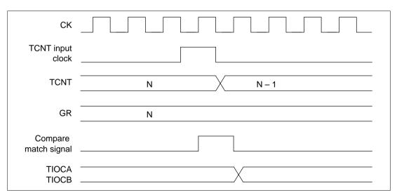
Figure 10.22 Compare Match Signal Output Timing
