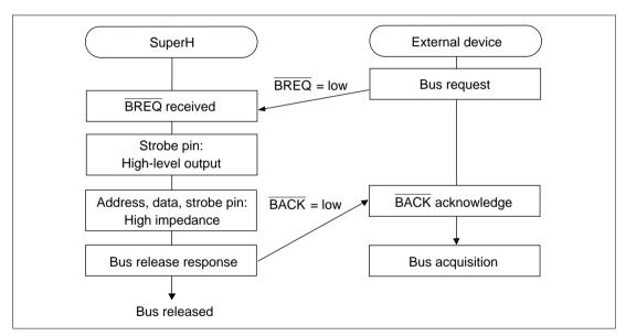
Figure 8.35 Bus Release Procedure
