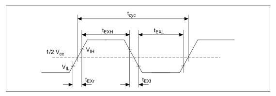
Figure 7.5 Input Clock Waveform
