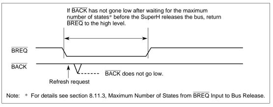
Figure 8.37 BACK Operation in Response to Refresh Request (2)
