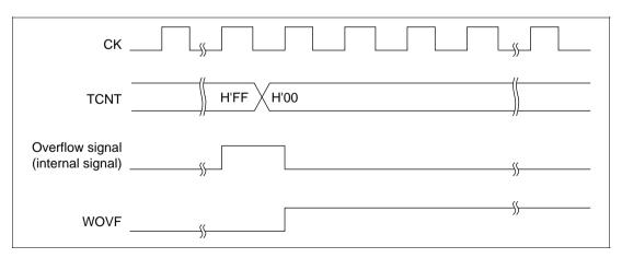
Figure 12.7 Timing of WOVF Bit Setting and Internal Reset
