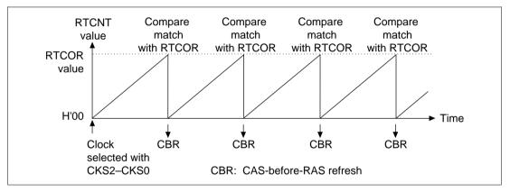
Figure 8.29 Refresh Timer Counter (RTCNT) Operation
