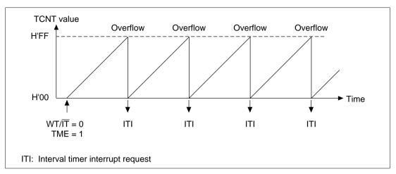
Figure 12.5 Operation in Interval Timer Mode
