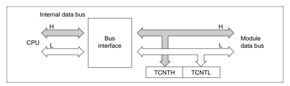
Figure 10.8 TCNT Access (CPU to TCNT (Upper Byte))
