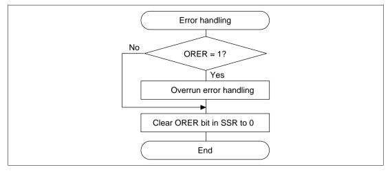
Figure 13.18 Sample Flowchart for Serial Receiving (cont)
