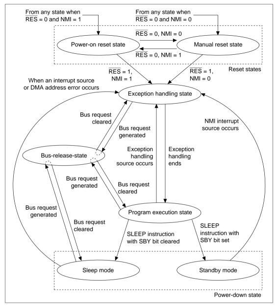
Figure 2.6 Transitions Between Processing States
