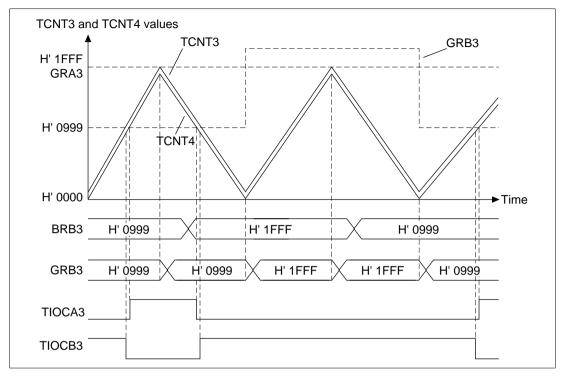
Figure 10.52 Buffer Mode Operation Example 3 (Complementary PWM Mode)
