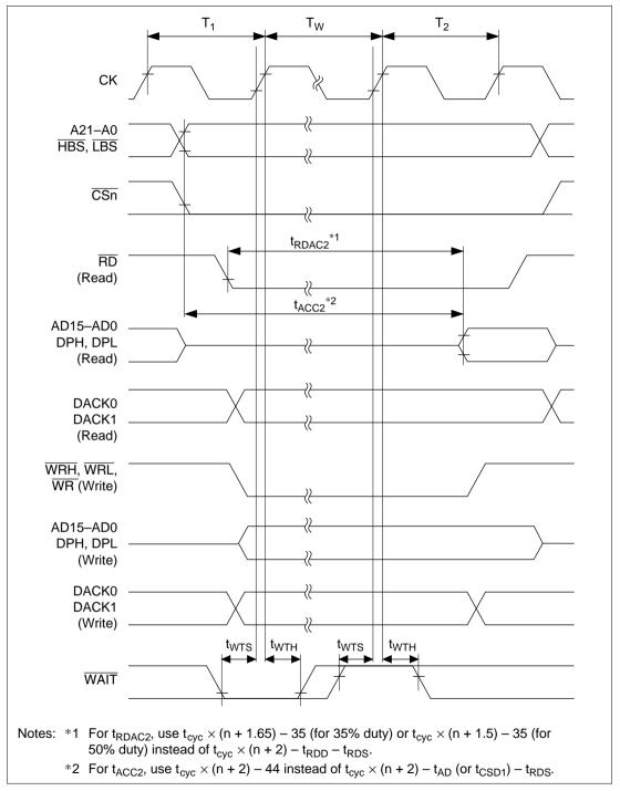
Figure 20.23 Basic Bus Cycle: Two States + Wait State
