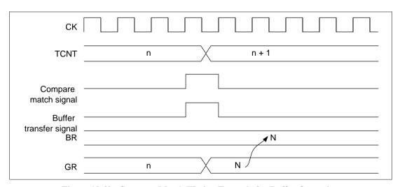
Figure 10.49 Compare Match Timing Example for Buffer Operation
