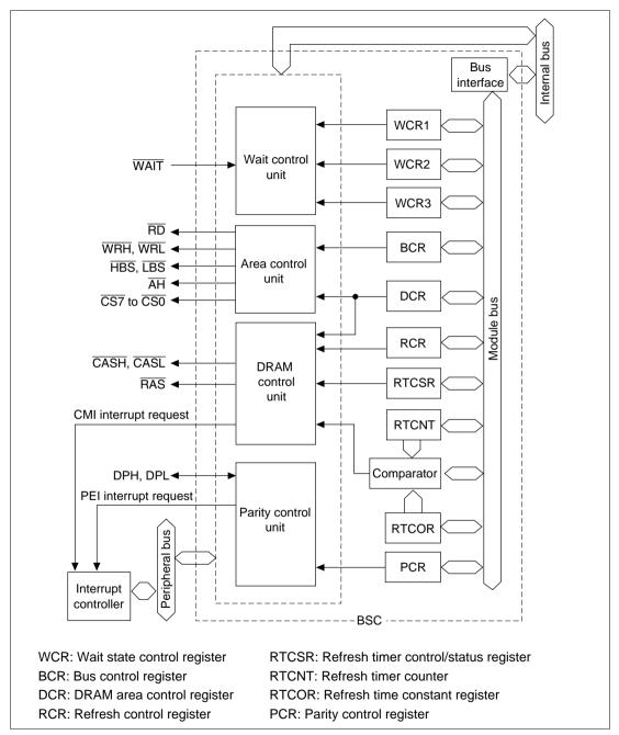
Figure 8.1 Block Diagram of BSC
