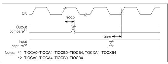
Figure 20.67 ITU Input/Output Timing
