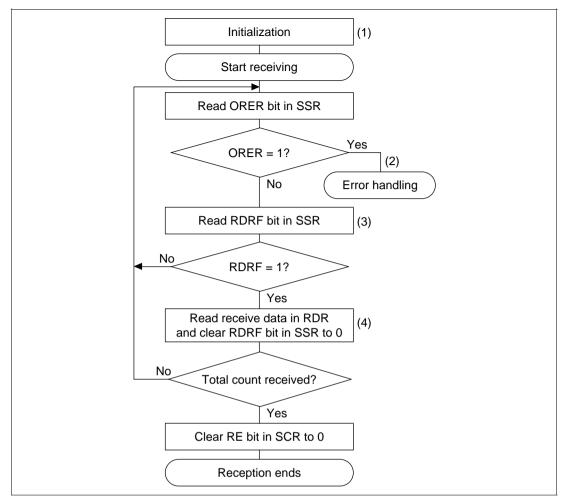
Figure 13.18 Sample Flowchart for Serial Receiving
