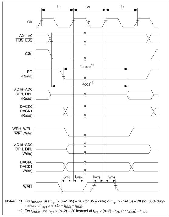
Figure 20.54 Basic Bus Cycle: Two States + Wait State
