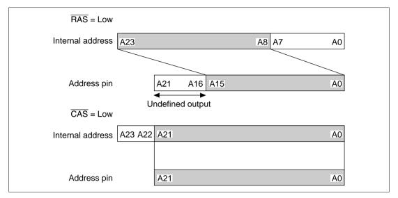
Figure 8.16 Address Multiplexing States (8-Bit Shift)
