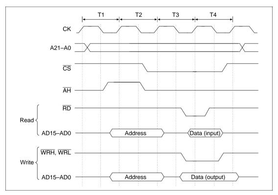
Figure 8.32 Access Timing For Address/Data Multiplexed I/O Space
