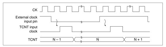
Figure 10.18 Count Timing for External Clock Sources (Both-Edge Detection)
