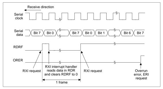
Figure 13.19 Example of SCI Receive Operation
