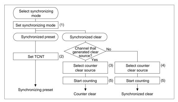
Figure 10.26 Procedure for Selecting Synchronizing Mode
