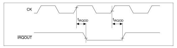
Figure 20.6 Interrupt Signal Output Timing
