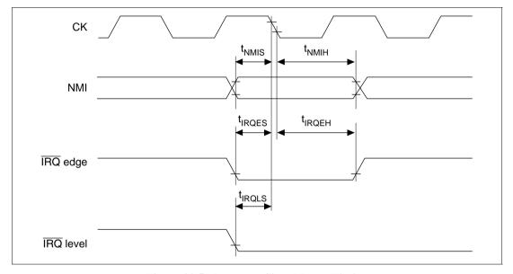
Figure 20.5 Interrupt Signal Input Timing
