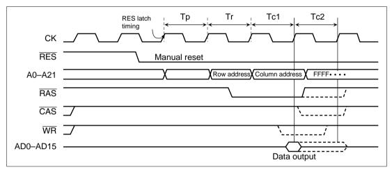
Figure 8.38 Long-Pitch Mode Write (1)
