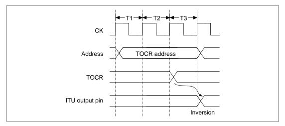
Figure 10.53 Example of Inverting ITU Output Levels by Writing to TOCR
