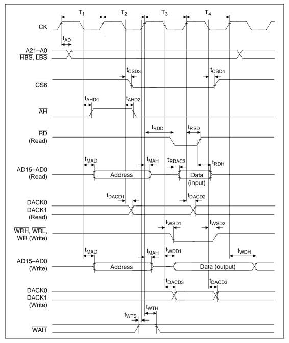
Figure 20.19 Address/Data Multiplex I/O Bus Cycle
