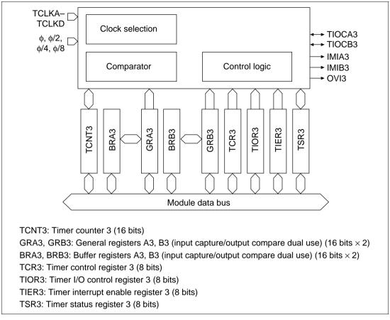
Figure 10.4 Block Diagram of Channel 3
