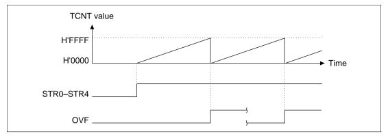
Figure 10.15 Free-Running Counter Operation
