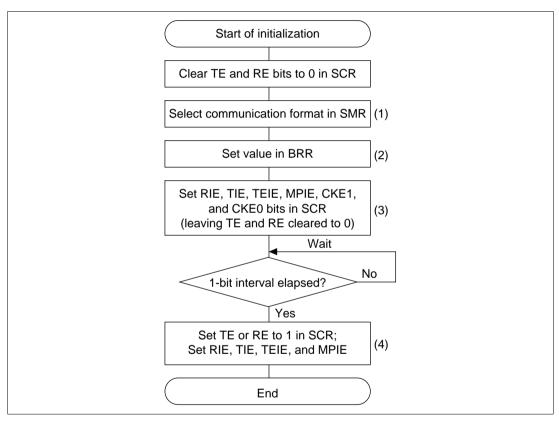
Figure 13.16 Sample Flowchart for SCI Initialization
