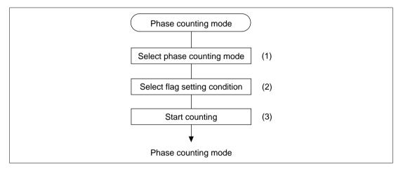
Figure 10.42 Procedure for Selecting Phase Counting Mode
