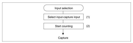
Figure 10.23 Procedure for Selecting Input Capture Mode
