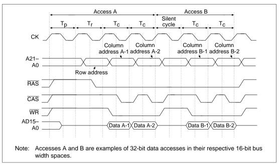
Figure 8.24 Short-Pitch, High-Speed Page Mode (Write Cycle)
