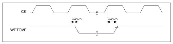
Figure 20.39 Watchdog Timer Output Timing
