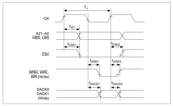
Figure 20.20 DMA Single Transfer/One-State Access Write
