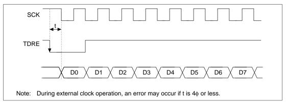
Figure 13.22 Example of Synchronous Transmitting with DMAC
