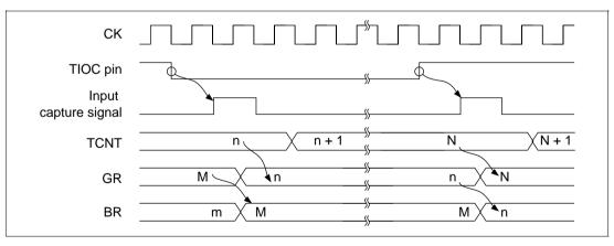
Figure 10.51 Input Capture Timing Example for Buffer Operation
