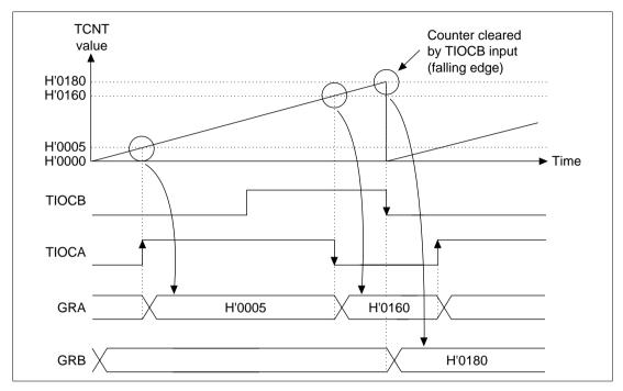
Figure 10.24 Input Capture Operation
