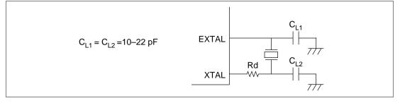
Figure 7.2 Connection of Crystal Resonator (Example)
