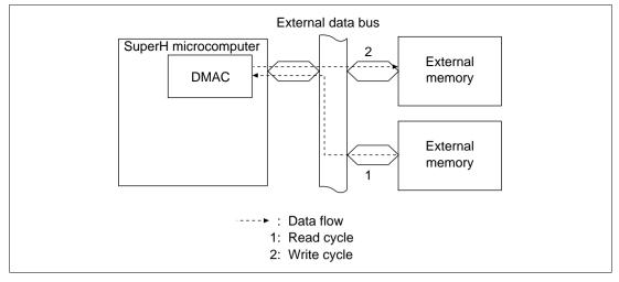
Figure 9.8 Data Flow in Dual Address Mode
