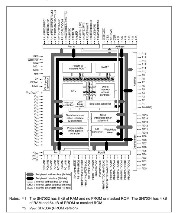
Figure 1.1 Block Diagram
