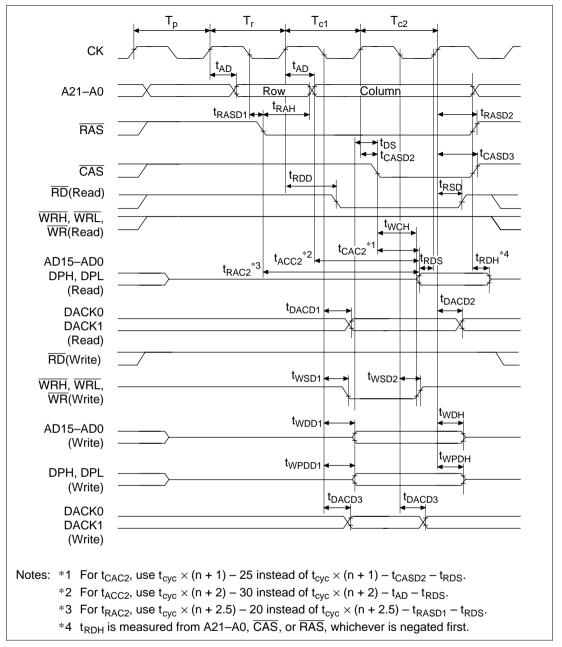
Figure 20.13 DRAM Bus Cycle: (Long-Pitch, Normal Mode)
