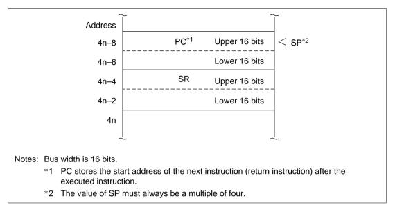
Figure 5.3 Stack after Interrupt Exception Handling
