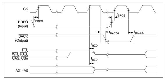
Figure 20.7 Bus Release Timing
