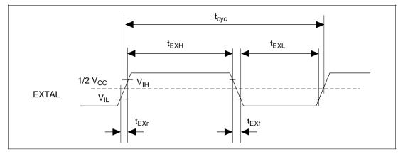
Figure 20.1 EXTAL Input Timing
