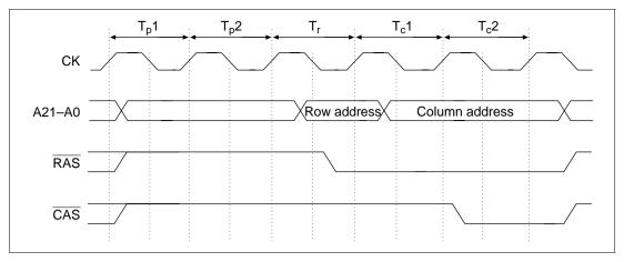
Figure 8.19 Precharge Timing (Long Pitch)
