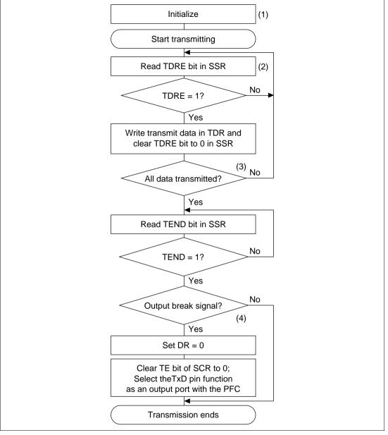
Figure 13.5 Sample Flowchart for Transmitting Serial Data
