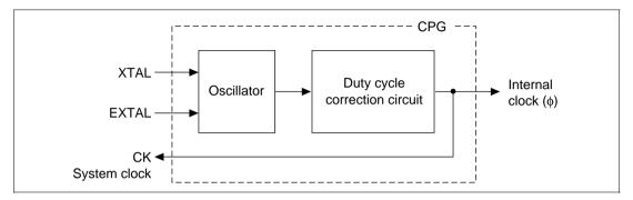
Figure 7.1 Block Diagram of Clock Pulse Generator
