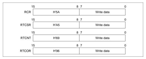
Figure 8.2 Writing to RCR, RTCSR, RTCNT, and RTCOR
