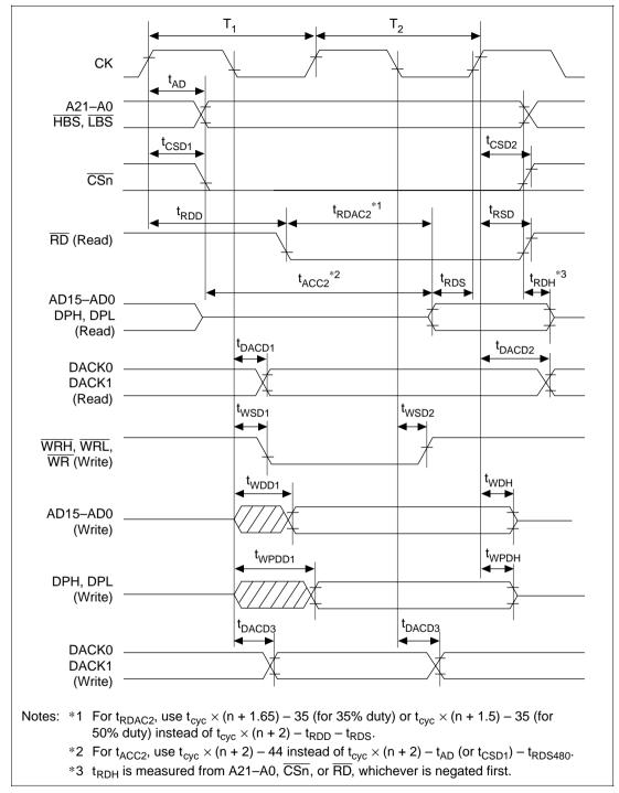
Figure 20.22 Basic Bus Cycle: Two-State Access
