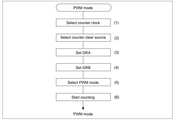
Figure 10.28 Procedure for Selecting PWM Mode
