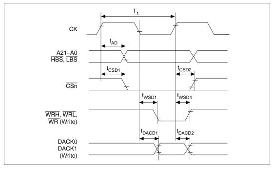
Figure 20.33 DMA Single Transfer/One-State Access Write
