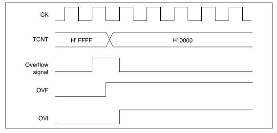
Figure 10.56 Timing of Setting OVF
