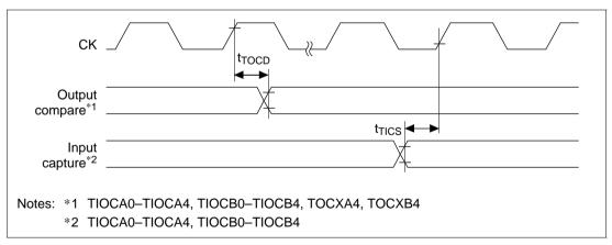
Figure 20.36 ITU Input/Output Timing
