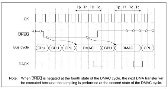
Figure 9.19 DREQ Sampling Timing in Cycle-Steal Mode (Output with DREQ Level Detection and DACK Active-Low) (Single Address Mode, Bus Cycle = DRAM Bus Cycle (Long Pitch Normal Mode))
