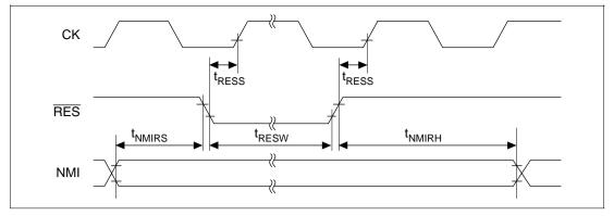
Figure 20.4 Reset Input Timing
