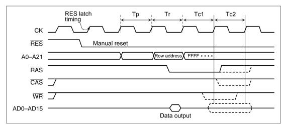
Figure 8.39 Long-Pitch Mode Write (2)
