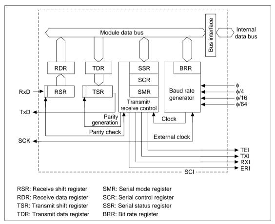
Figure 13.1 Block Diagram of SCI
