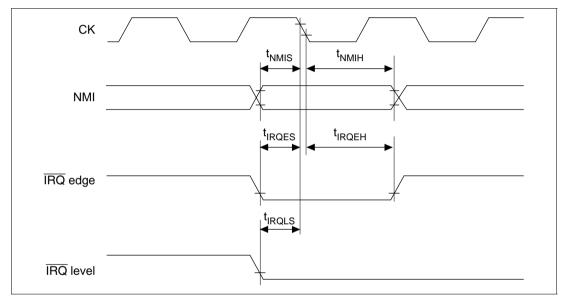
Figure 20.49 Interrupt Signal Input Timing
