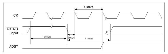
Figure 20.73 External Trigger Input Timing
