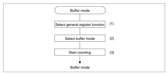
Figure 10.47 Procedure for Selecting Buffer Mode
