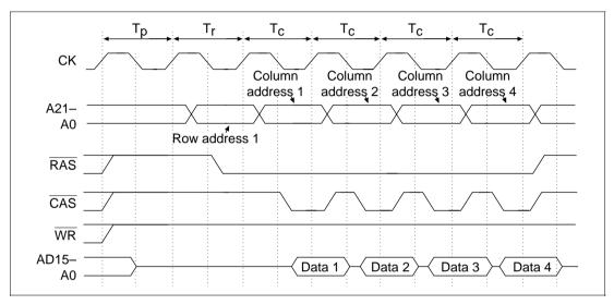
Figure 8.23 Short-Pitch, High-Speed Page Mode (Read Cycle)
