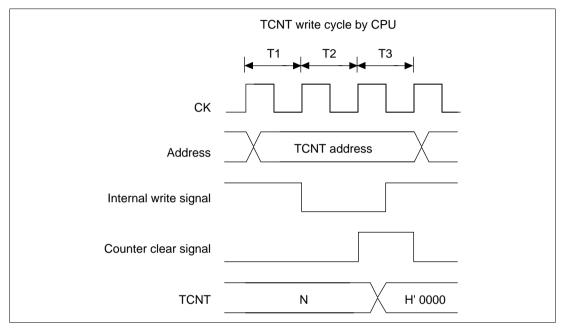
Figure 10.58 Contention between TCNT Write and Clear
