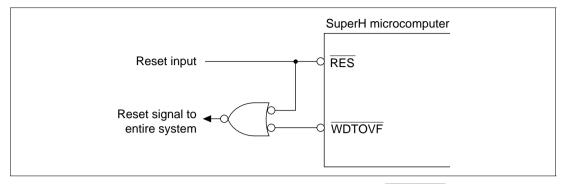
Figure 12.9 Example of System Reset Circuit Using WDTOVF Signal
