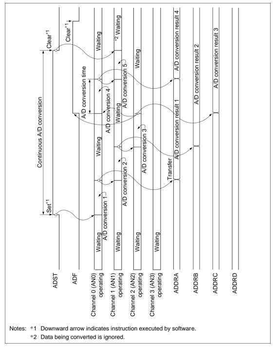
Figure 14.4 A/D Operation in Scan Mode (Channels 0-2 Selected)
