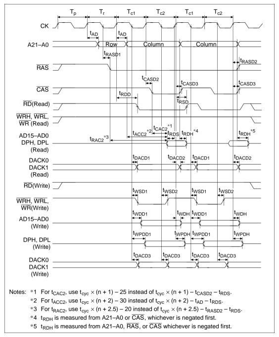
Figure 20.14 DRAM Bus Cycle: (Long-Pitch, High-Speed Page Mode)
