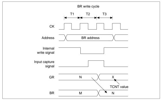
Figure 10.66 Contention between BR Write and Input Capture
