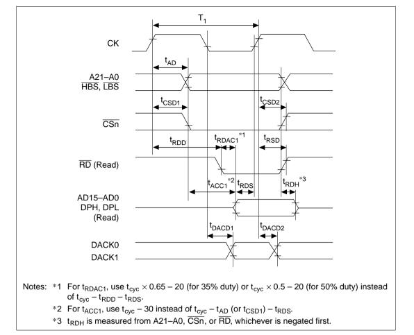
Figure 20.8 Basic Bus Cycle: One-State Access
