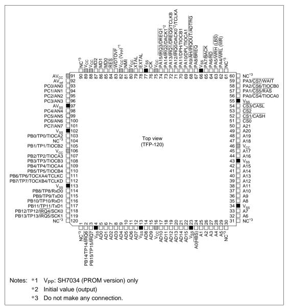
Figure 1.3 Pin Arrangement (TFP-120)
