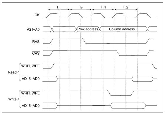
Figure 8.18 Long Pitch Access Timing
