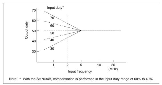
Figure 7.7 Duty Cycle Correction Circuit Standard Characteristics
