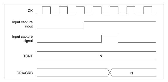
Figure 10.25 Input Capture Signal Timing
