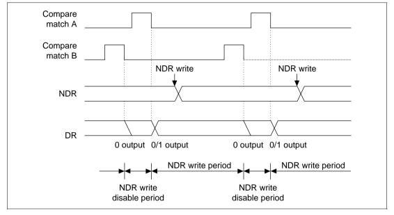
Figure 11.10 Non-Overlap Operation and NDR Write Timing
