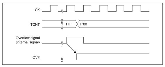
Figure 12.6 Timing of OVF Setting
