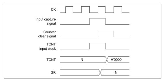
Figure 10.64 Contention between Counter Clearing by Input Capture and Counter Increment
