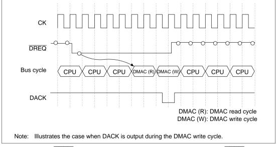
Figure 9.16 DREQ Sampling Timing in Cycle-Steal Mode (Output with DREQ Level Detection and DACK Active-Low) (Dual Address Mode, Bus Cycle = 2 States)
