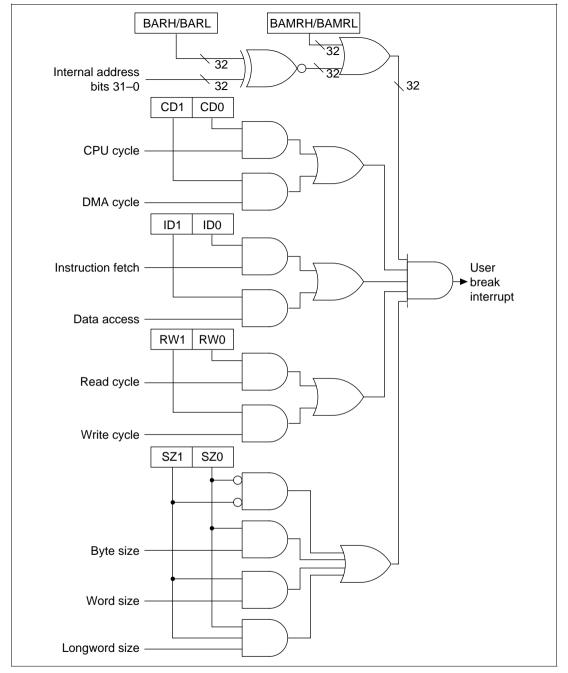
Figure 6.2 Break Condition Logic
