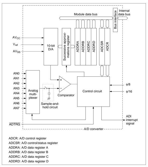
Figure 14.1 Block Diagram of A/D Converter
