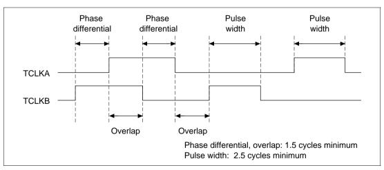
Figure 10.44 Phase Differentials, Overlap, and Pulse Width in Phase Counting Mode
