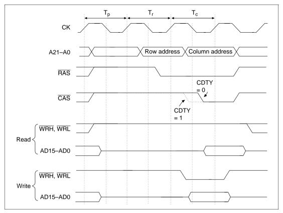
Figure 8.17 Short Pitch Access Timing
