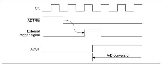
Figure 14.6 External Trigger Input Timing
