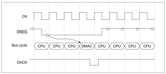
Figure 9.13 DREQ Sampling Timing in Cycle-Steal Mode (Output with DREQ Level Detection and DACK Active-Low) (Single Address Mode, Bus Cycle = 1 State)
