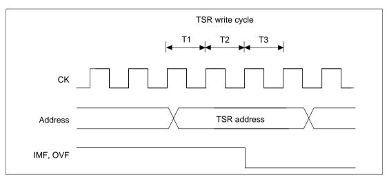
Figure 10.57 Timing of Status Flag Clearing
