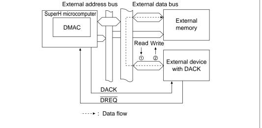
Note: The read/write direction is decided by the RS3-RS0 bits in the CHCRn registers. If RS3-RS0 = 0010, the direction is as shown in case 1 (circled number above); if RS3-RS0 = 0011, the direction is as shown in case 2. In the Electrical Characteristics section, DACK output (read) indicates case 1, and DACK output (write) indicates case 2.
