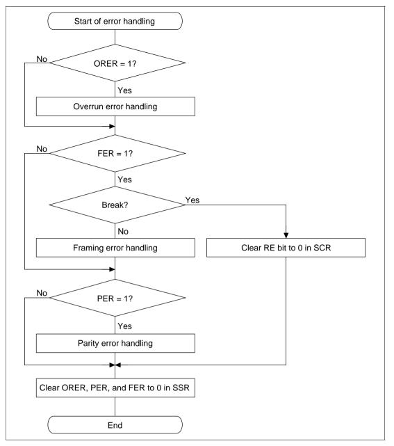
Figure 13.7 Sample Flowchart for Receiving Serial Data (cont)
