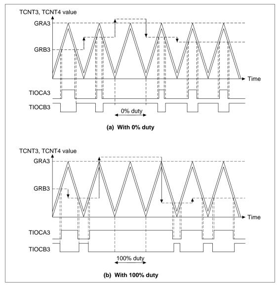
Figure 10.35 Complementary PWM Mode Operation Example 2
