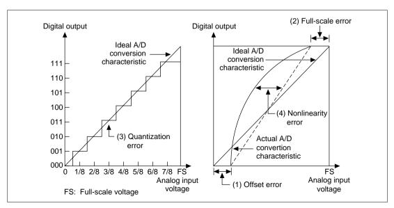
Figure 14.7 Definitions of A/D Conversion Accuracy
