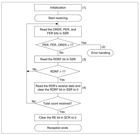
Figure 13.7 Sample Flowchart for Receiving Serial Data
