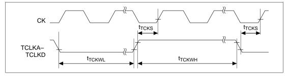
Figure 20.37 ITU Clock Input Timing
