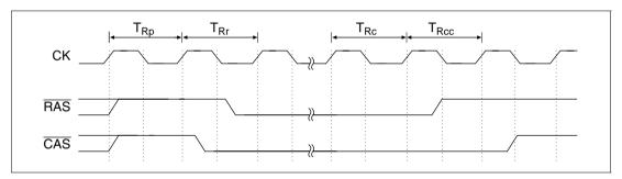
Figure 8.31 Output Timing for Self-Refresh Signal
