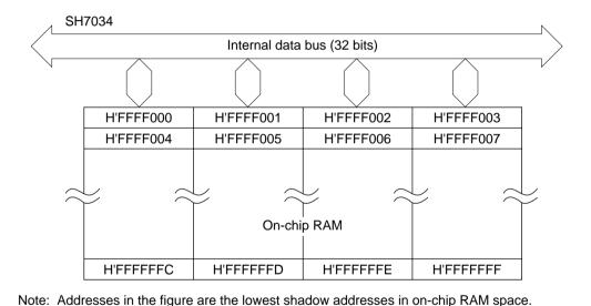
Figure 18.1 Block Diagram of RAM
