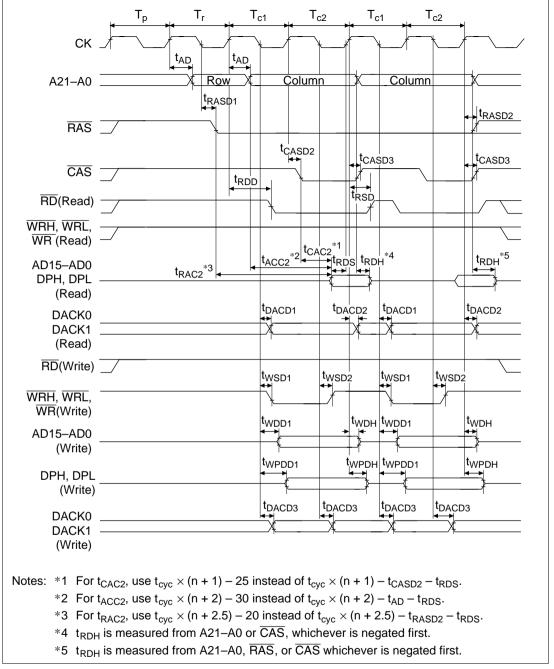
Figure 20.58 DRAM Bus Cycle: (Long-Pitch, High-Speed Page Mode)
