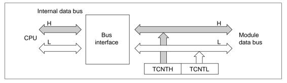
Figure 10.10 TCNT Access (TCNT to CPU (Upper Byte))
