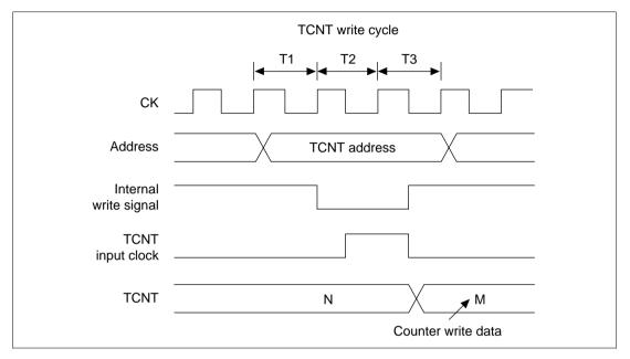
Figure 12.8 Contention between TCNT Write and Increment
