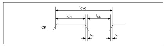
Figure 20.2 System Clock Timing
