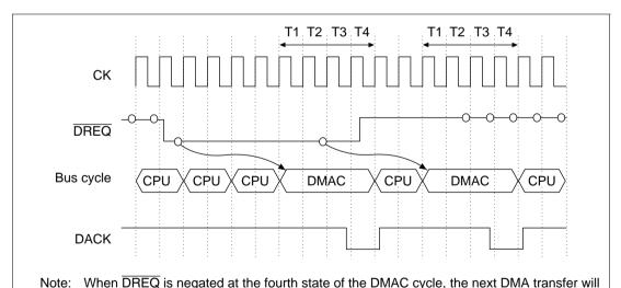
Figure 9.21 DREQ Sampling Timing in Cycle-Steal Mode (Output with DREQ Level Detection and DACK Active-Low) (Single Address Mode, Bus Cycle = Address/Data **Multiplex I/O Bus Cycle)**
