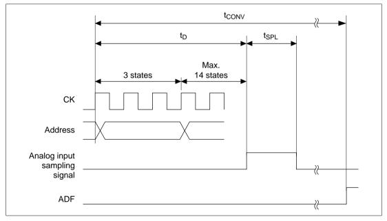
Figure 20.74 Analog Conversion Timing
