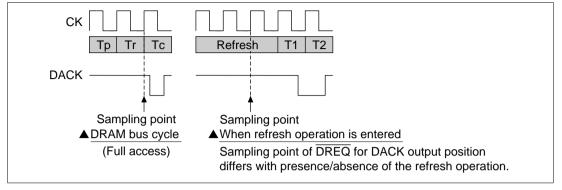
Figure 9.26 Example of DREQ Sampling before Output of DACK
