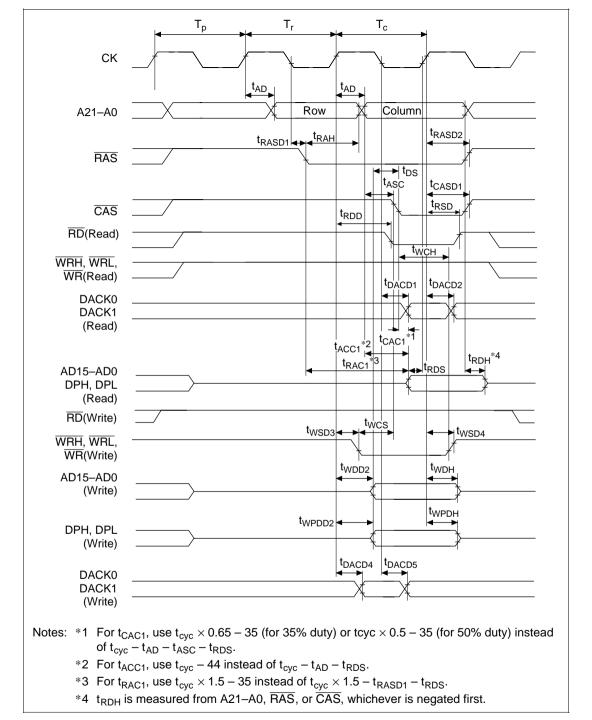
Figure 20.24 DRAM Bus Cycle (Short-Pitch, Normal Mode)
