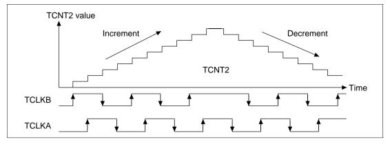
Figure 10.43 Phase Counting Mode Operation
