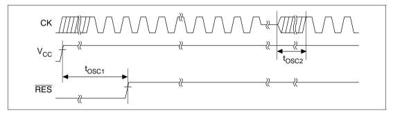
Figure 20.3 Oscillation Settling Time
