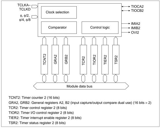
Figure 10.3 Block Diagram of Channel 2
