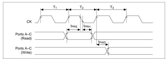
Figure 20.38 Programmable Timing Pattern Controller Output Timing
