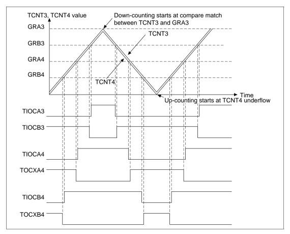
Figure 10.34 Complementary PWM Mode Operation Example 1
