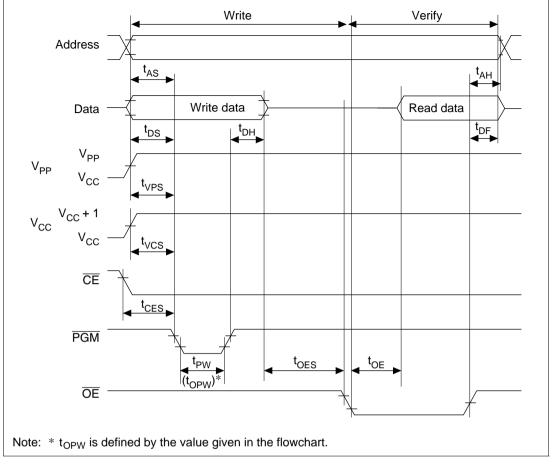
Figure 17.5 Write/Verify Timing
