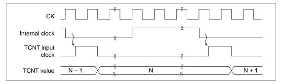
Figure 10.17 Count Timing for Internal Clock Sources
