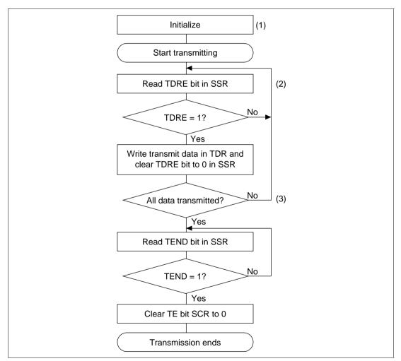
Figure 13.17 Sample Flowchart for Serial Transmitting
