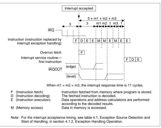
Figure 5.4 Example of Pipelining in IRQ Interrupt Acceptance
