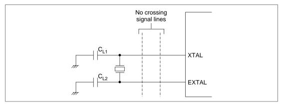
Figure 7.6 Precaution on Oscillator Circuit Board Design
