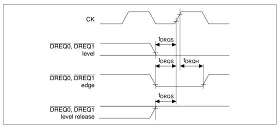
Figure 20.65 DREQ0, DREQ1 Input Timing (1)
