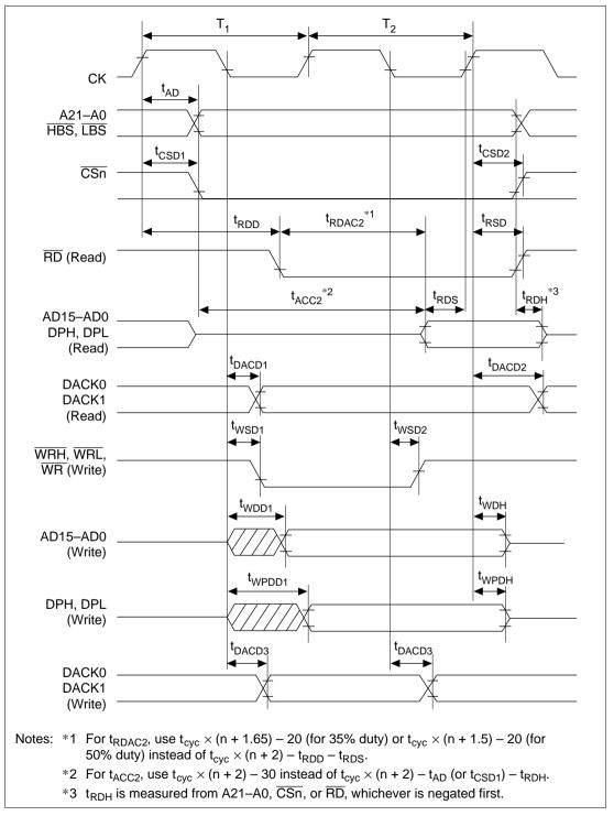
Figure 20.53 Basic Bus Cycle: Two-State Access
