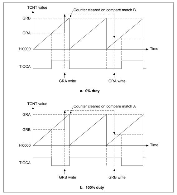
Figure 10.30 PWM Mode Operation Example 2
