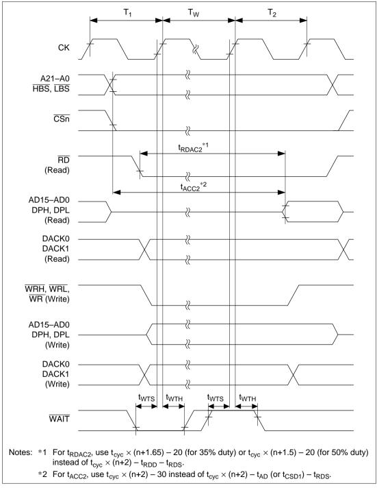
Figure 20.10 Basic Bus Cycle: Two States + Wait State
