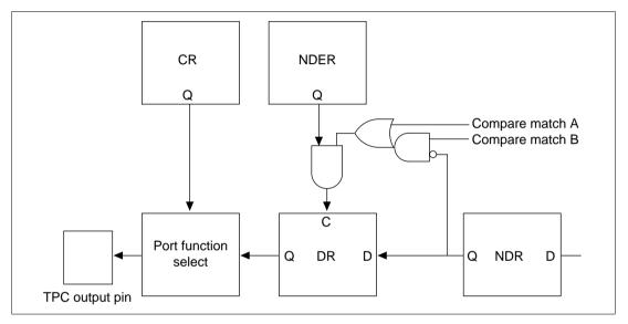
Figure 11.9 TPC Output Non-Overlap Operation
