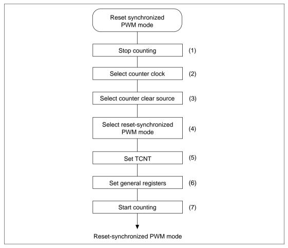
Figure 10.31 Procedure for Selecting Reset-Synchronized PWM Mode
