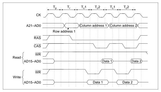
Figure 8.26 Long-Pitch, High-Speed Page Mode (Read/Write Cycle)
