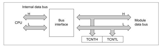
Figure 10.6 TCNT Access (CPU to TCNT (Word))
