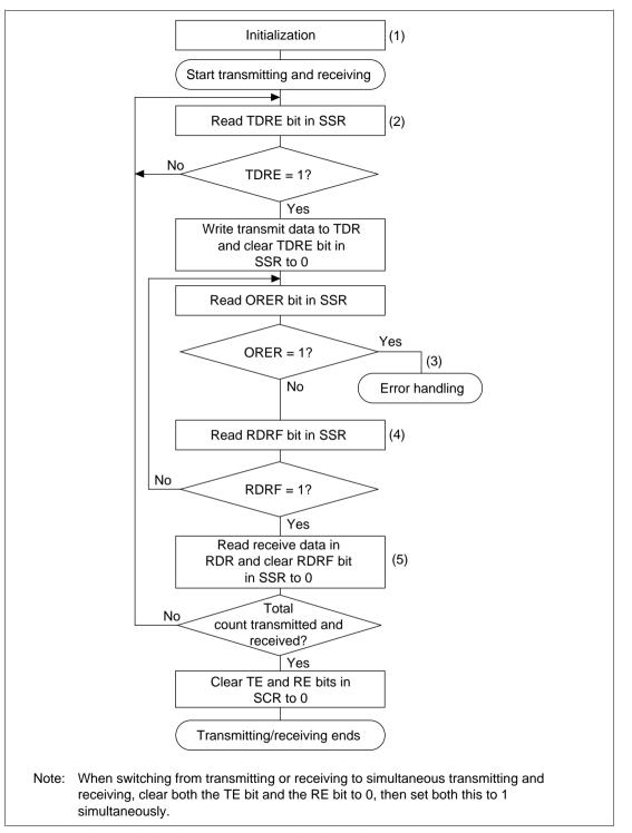
Figure 13.20 Sample Flowchart for Serial Transmitting and Receiving
