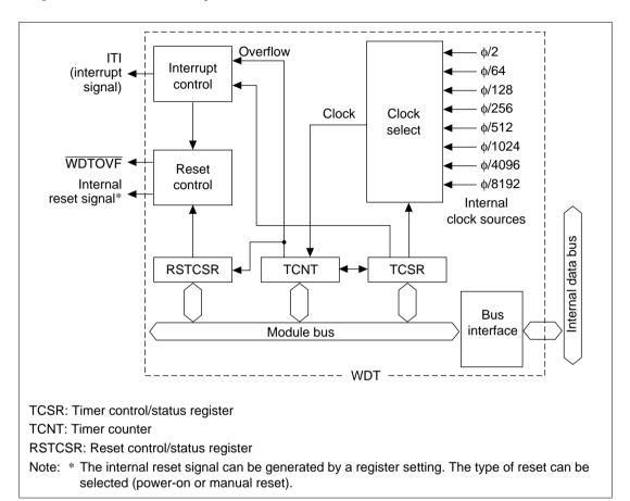
Figure 12.1 Block Diagram of WDT
