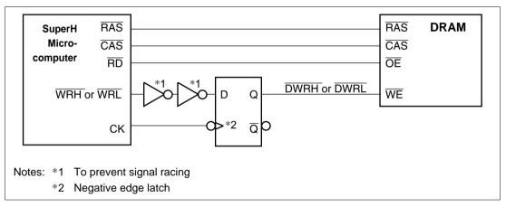
Figure 8.42 Delayed-Write Control Circuit
