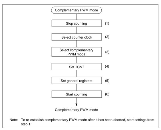
Figure 10.33 Procedure for Selecting Complementary PWM Mode
