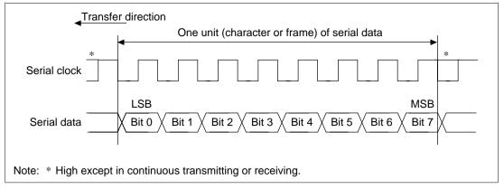
Figure 13.14 Data Format in Synchronous Communication
