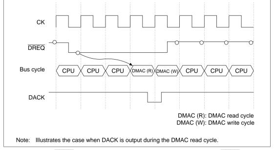
Figure 9.14 DREQ Sampling Timing in Cycle-Steal Mode (Output with DREQ Level Detection and DACK Active-Low) (Dual Address Mode, Bus Cycle = 1 State)
