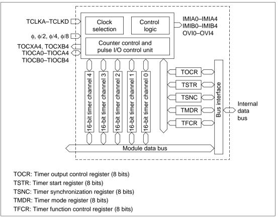
Figure 10.1 Block Diagram of ITU
