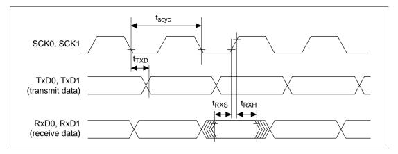
Figure 20.72 SCI I/O Timing (Synchronous Mode)
