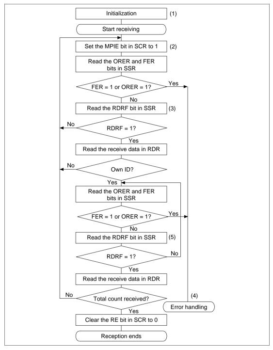
Figure 13.12 Sample Flowchart for Receiving Multiprocessor Serial Data
