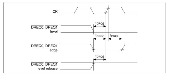
Figure 20.34 DREQ0, DREQ1 Input Timing (1)
