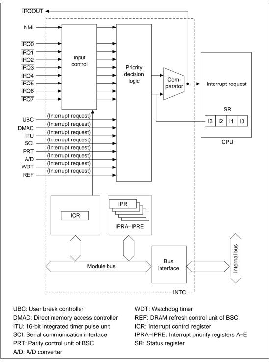
Figure 5.1 Block Diagram of Interrupt Controller
