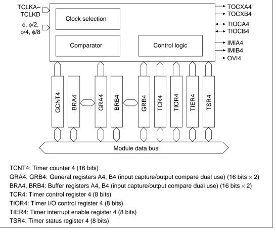
Figure 10.5 Block Diagram of Channel 4
