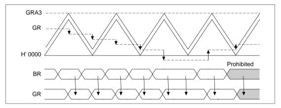
Figure 10.38 Example of Changing GR Settings with Buffer Operation (1)
