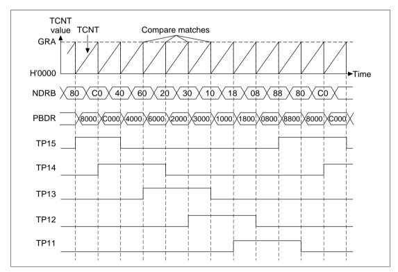
Figure 11.5 TPC Output Example (5-Phase Pulse Output)
