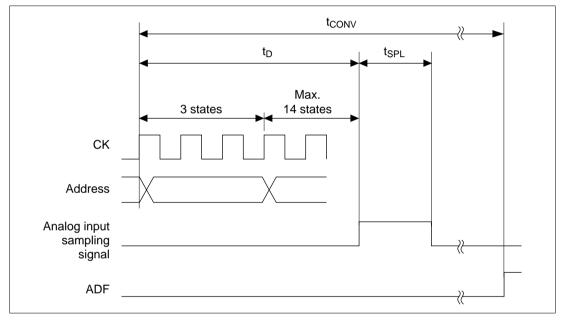
Figure 20.43 Analog Conversion Timing
