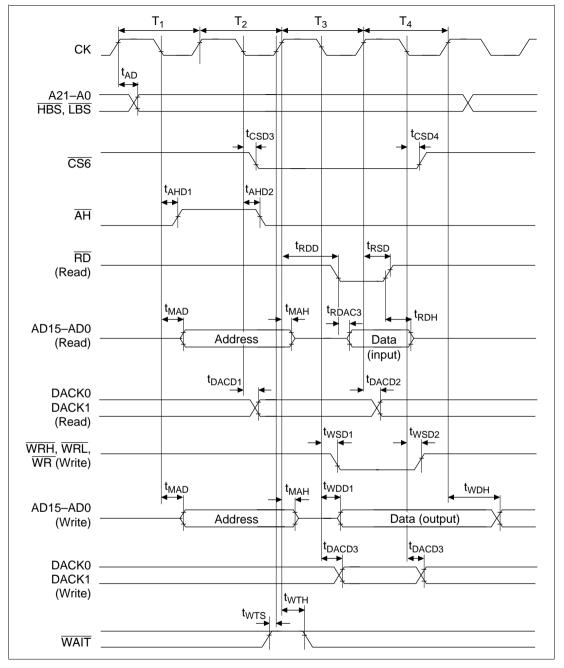
Figure 20.63 Address/Data Multiplex I/O Bus Cycle
