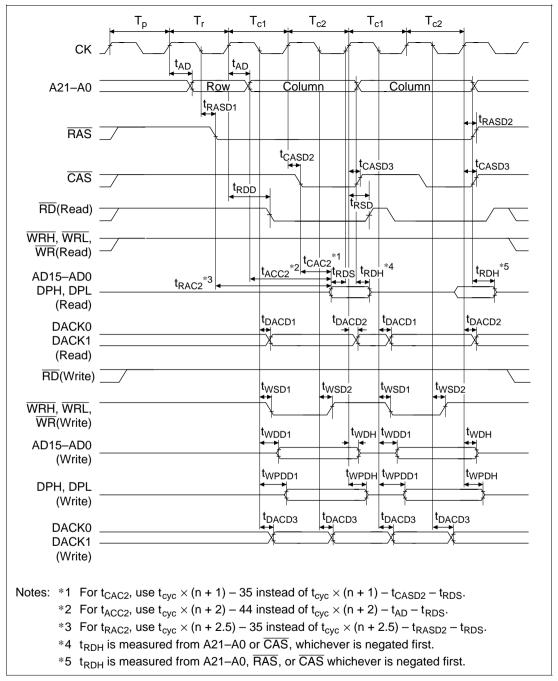
Figure 20.27 DRAM Bus Cycle: (Long-Pitch, High-Speed Page Mode)
