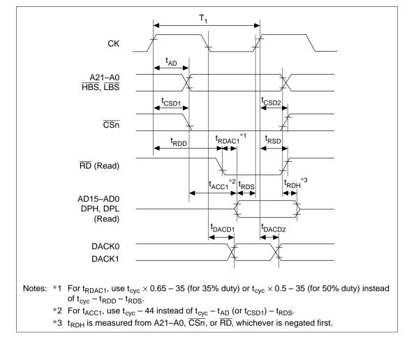
Figure 20.21 Basic Bus Cycle: One-State Access
