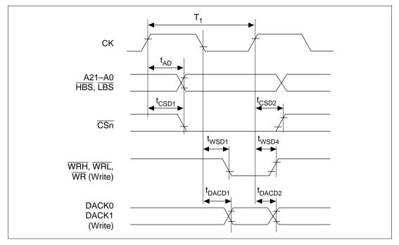
Figure 20.64 DMA Single Transfer/One-State Access Write
