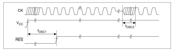
Figure 20.47 Oscillation Settling Time
