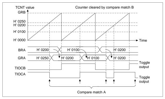
Figure 10.48 Buffer Mode Operation Example 1 (Output Compare Register)
