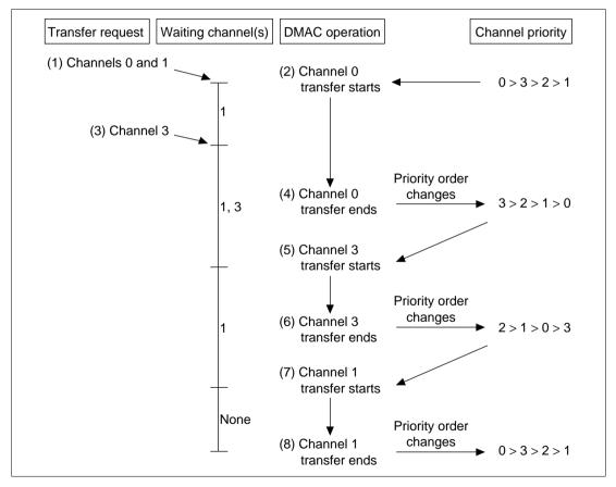
Figure 9.4 Changes in Channel Priority in Round-Robin Mode
