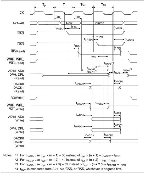
Figure 20.26 DRAM Bus Cycle: (Long-Pitch, Normal Mode)
