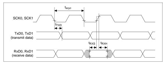
Figure 20.41 SCI I/O Timing (Synchronous Mode)
