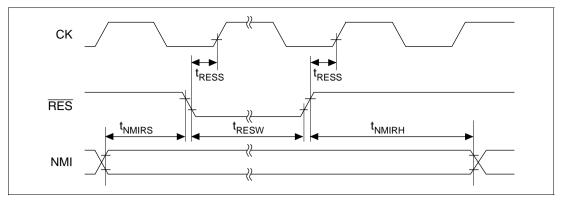
Figure 20.48 Reset Input Timing
