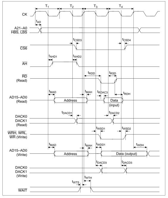
Figure 20.32 Address/Data Multiplex I/O Bus Cycle
