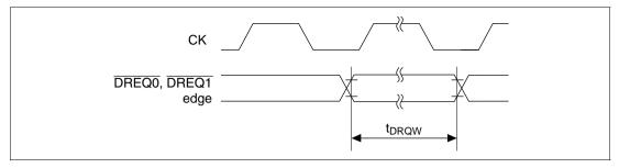
Figure 20.66 DREQ0, DREQ1 Input Timing (2)
