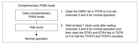
Figure 10.69 Clearing Complementary PWM Mode
