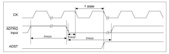
Figure 20.42 External Trigger Input Timing
