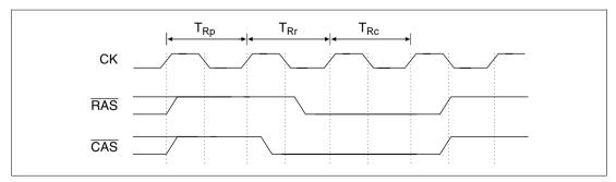
Figure 8.30 Output Timing for CAS-Before-RAS Refresh Signal
