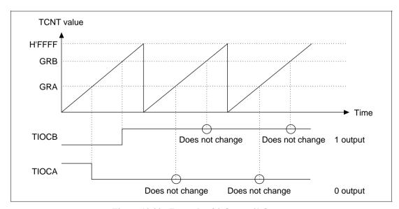
Figure 10.20 Example of 0 Output/1 Output
