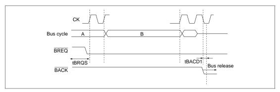
Figure 8.43 When  $\overline{BREQ}$  is Input without Satisfying tBRQS
