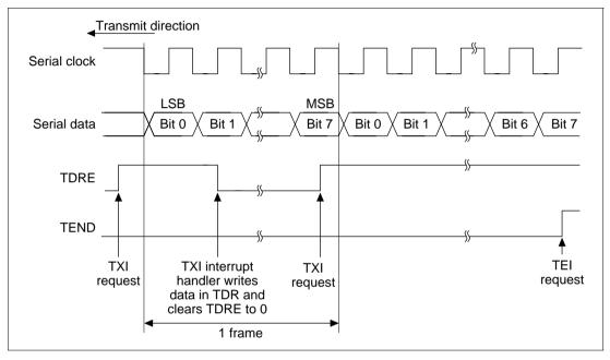
Figure 13.15 Example of SCI Transmit Operation
