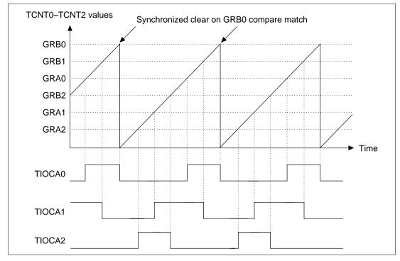
Figure 10.27 Example of Synchronized Operation
