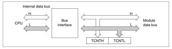
Figure 10.9 TCNT Access (CPU to TCNT (Lower Byte))
