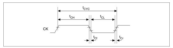
Figure 20.46 System Clock Timing
