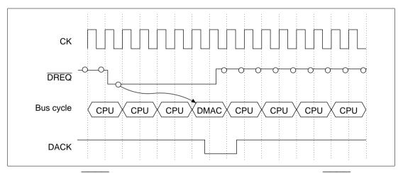
Figure 9.15 DREQ Sampling Timing in Cycle-Steal Mode (Output with DREQ Level Detection and DACK Active-Low) (Single Address Mode, Bus Cycle = 2 States)
