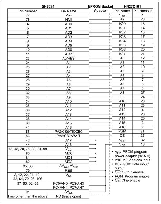
Figure 17.2 Correspondence Between SH7034 Pins and HN27C101 Pins
