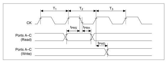
Figure 20.69 Programmable Timing Pattern Controller Output Timing
