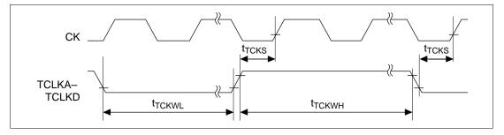
Figure 20.68 ITU Clock Input Timing
