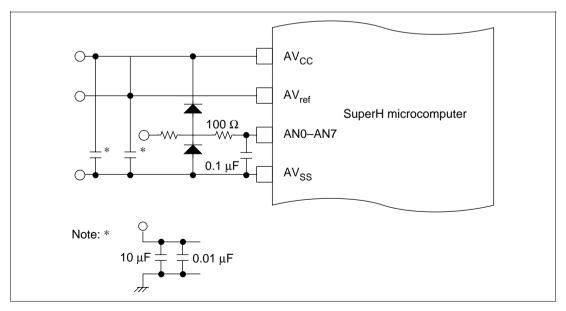
Figure 14.8 Example of Analog Input Protection Circuit
