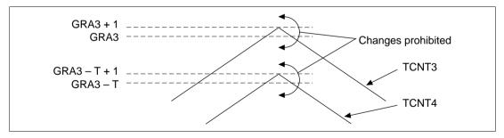
Figure 10.39 Caution on Changing GR Settings with Buffer Operation (1)
