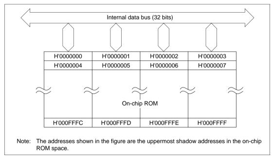
Figure 17.1 Block Diagram of ROM
