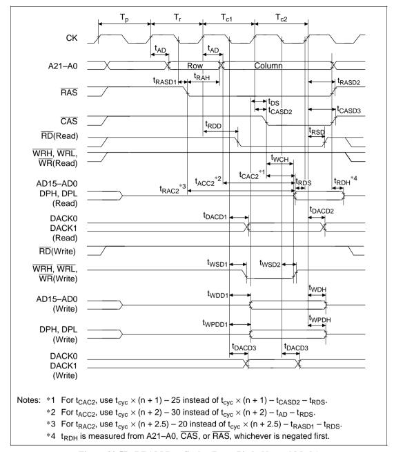
Figure 20.57 DRAM Bus Cycle: (Long-Pitch, Normal Mode)
