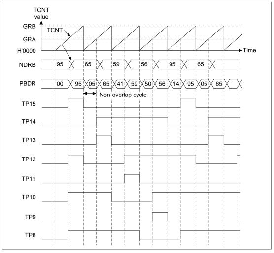
Figure 11.7 Non-Overlap Output Example (Four-Phase Complementary Output)
