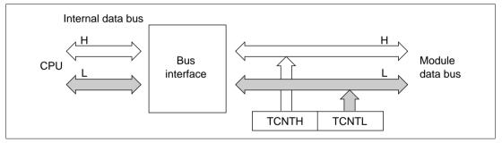
Figure 10.11 TCNT Access (TCNT to CPU (Lower Byte))
