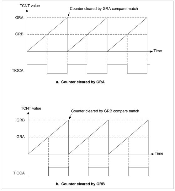
Figure 10.29 PWM Mode Operation Example 1
