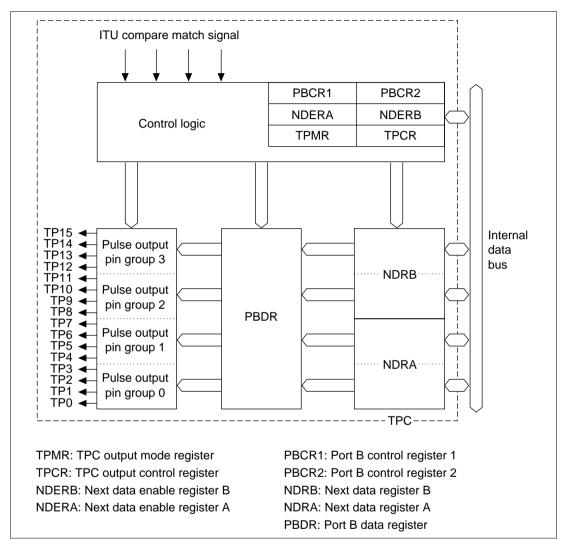
Figure 11.1 Block Diagram of TPC
