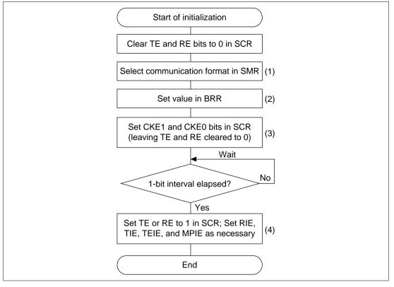
Figure 13.4 Sample Flowchart for SCI Initialization
