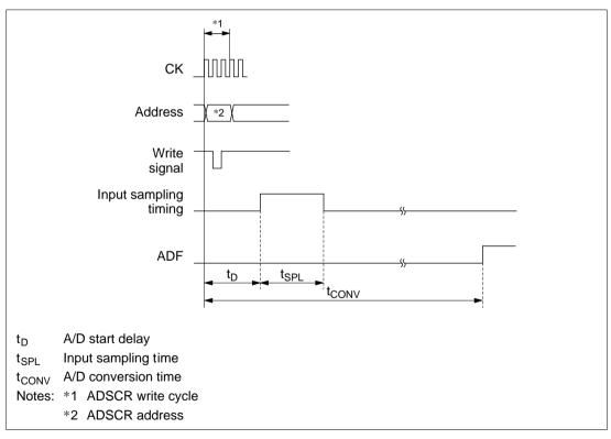
Figure 14.5 A/D Conversion Timing
