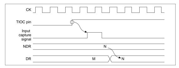
Figure 11.8 TPC Output by Input Capture
