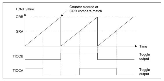
Figure 10.21 Example of Toggle Output
