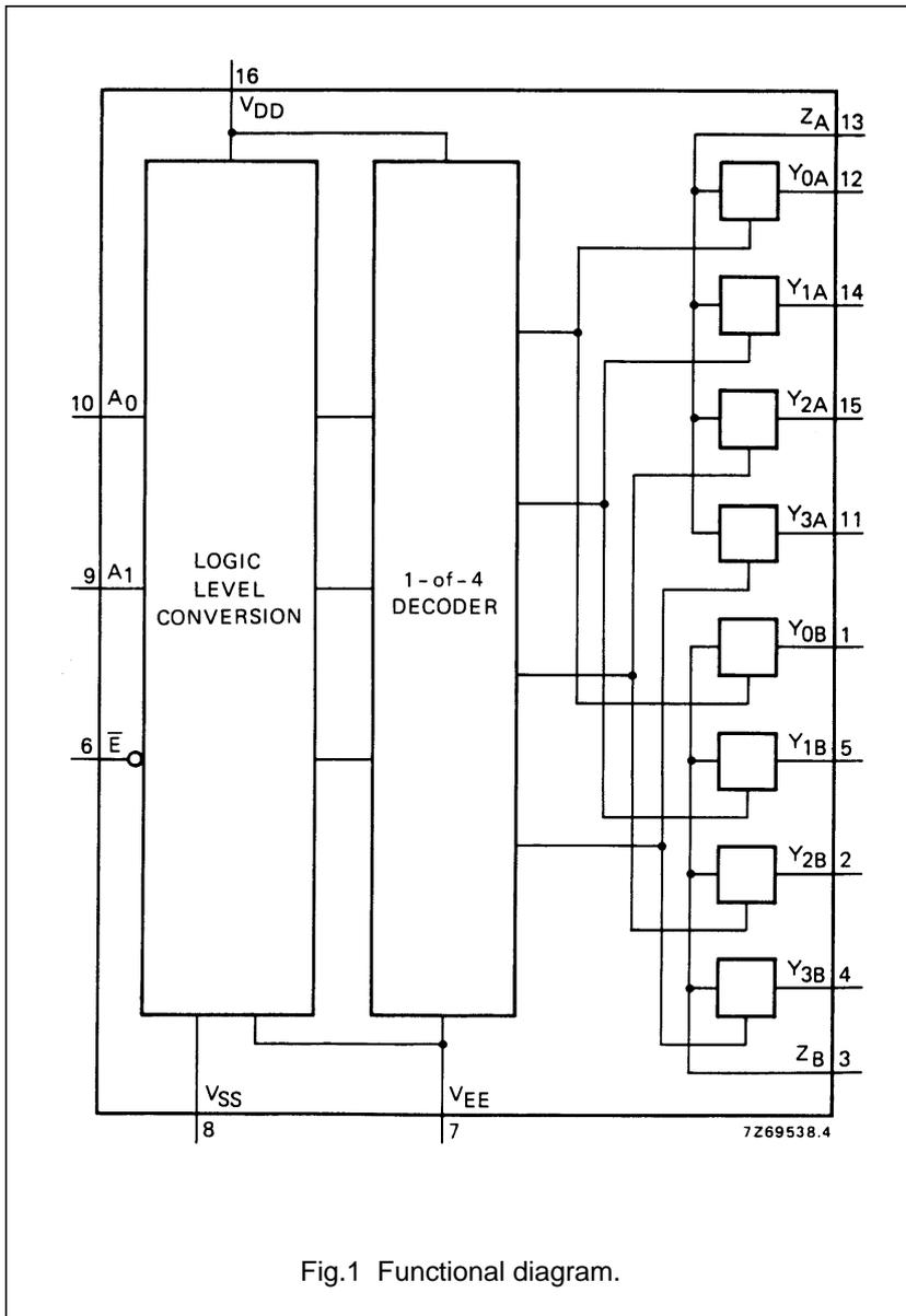
Fig.1 Functional diagram.
