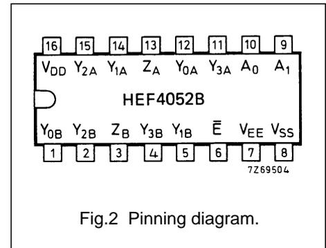
Fig.2 Pinning diagram.
