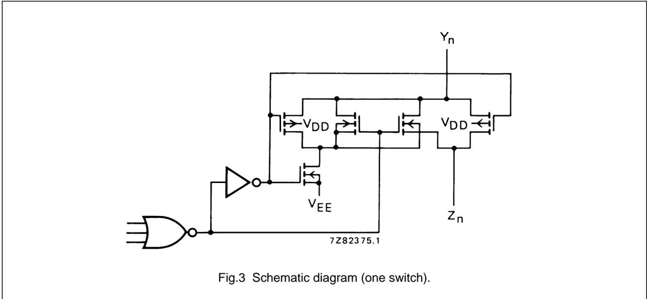
Fig.3 Schematic diagram (one switch).
