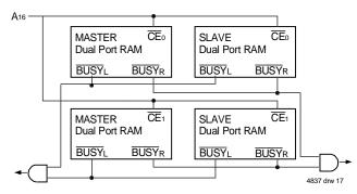
Figure 3. Busy and chip enable routing for both width and depth expansion with IDT7038 RAMs.
