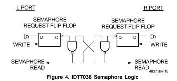
over to the other side as soon as a one is written into the first side's request latch. The second side's flag will now stay LOW until its semaphore request latch is written to a one. From this it is easy to understand that, if a semaphore is requested and the processor which requested it no longer needs the resource, the entire system can hang up until a one is written into that semaphore request latch.
