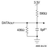
Figure 1. AC Output Load
