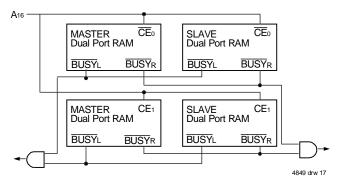
Figure 3. Busy and chip enable routing for both width and depth expansion with IDT70V28 RAMs.
