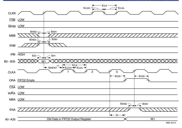
Figure 10. ORA Flag Timing and First Data Word Fall Through when FIFO2 is Empty (FWFT Mode)
