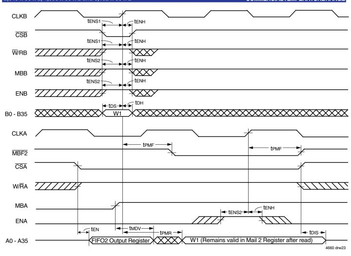
Figure 21. Timing for Mail2 Register and MBF2 Flag (IDT Standard and FWFT Modes)
