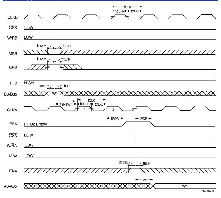
Figure 11. EFA Flag Timing and First Data Read when FIFO2 is Empty (IDT Standard Mode)
