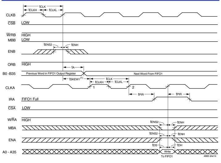
Figure 12. IRA Flag Timing and First Available Write when FIFO1 is Full (FWFT Mode)
