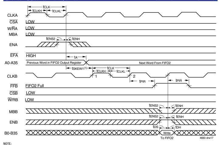
1. tskew1 is the minimum time between a rising CLKA edge and a rising CLKA edge for FFB to transition HIGH in the next CLKB cycle. If the time between the rising CLKA edge and rising CLKB edge is less than tskew1, then FFB may transition HIGH one CLKB cycle later than shown.
