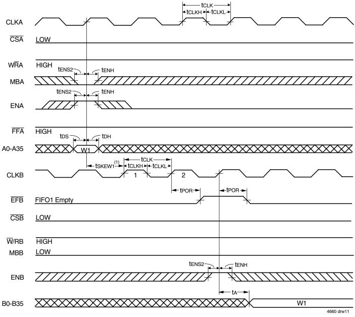
Figure 9. EFB Flag Timing and First Data Read Fall Through when FIFO1 is Empty (IDT Standard Mode)
