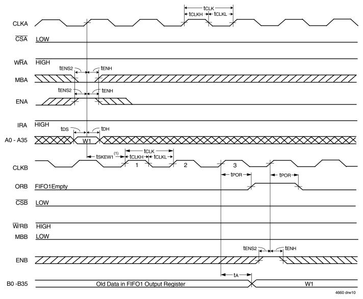
Figure 8. ORB Flag Timing and First Data Word Fall Through when FIFO1 is Empty (FWFT Mode)
