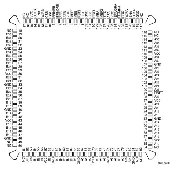
Electrical pin 1 in center of beveled edge. Pin 1 identifier in corner.
