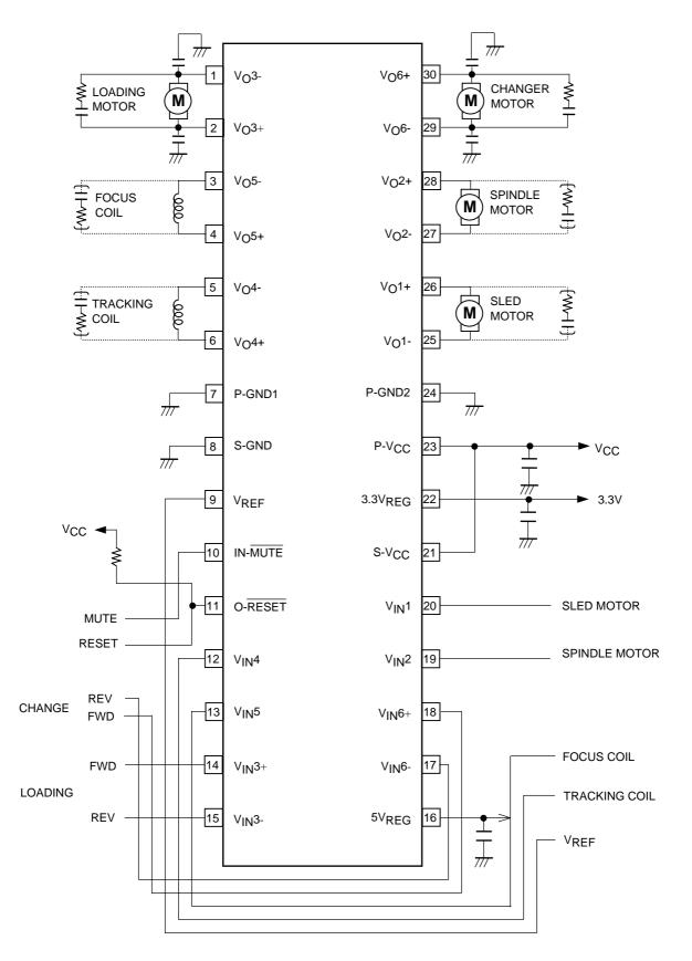
Note: When connecting a load to CH3 and CH6, set the output capacitor to  $0.56\mu$ F or more and select the capacitor according to the setting. The capacitor to be used should be less in capacity fluctuation due to temperature.
