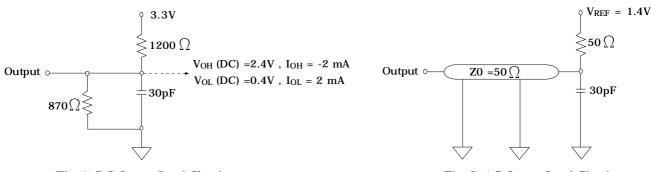
(Fig. 1) DC Output Load Circuit
