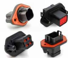
The Amphenol Panel | Mate™ series combines flange mounting options with the proven reliability of the AT/ATP Series™ environmentally-sealed thermoplastic connection system. Engineered with a one-piece sealed flange design for rapid and secure mounting, its durable high temperature silicone facial seal provides a barrier of protection from lubricating oils, hydraulic fluids and fossil fuels to withstand the challenges and complexities of harsh environment applications.
