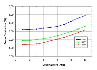
Figure 4. Power dissipation vs. load current and input voltage for SSQE48T10033 converter mounted vertically with air flowing from pin 1 to pin 3at a rate of 300 LFM (1.5 m/s) and Ta = 25 °C.
