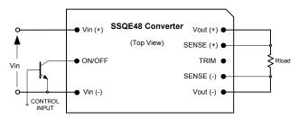
Fig. A: Circuit configuration for ON/OFF function.
