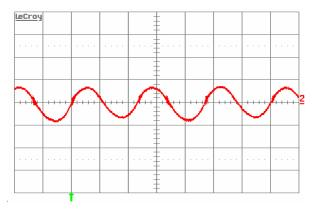
Figure 13. Input reflected ripple-current, i<sub>c</sub> (100 mA/div.), measured at input terminals at full rated load current and Vin = 48 V. Refer to Figure 11 for test setup. Time scale: 1 μs/div.
