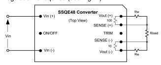
Fig. B: Remote sense circuit configuration.
