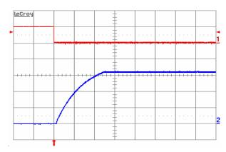
Figure 7. Turn-on transient at full rated load current (resistive) plus 20,000  $\mu$ F at Vin = 48 V, triggered via ON/OFF pin. Top trace: ON/OFF signal (5 V/div.). Bottom trace: Output voltage (1 V/div.). Time scale: 5 ms/div.
