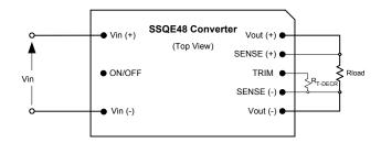
Fig. D: Configuration for decreasing output voltage.
