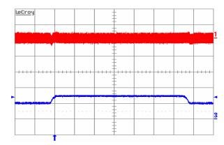
Figure 8. Output voltage response to load current stepchange (5A-7.5A-5A) at Vin=48V. Top trace: output voltage (50 mV/div.). Bottom trace: load current (5A/div.). Current slew rate: 0.1A/μs. Co=1μF ceramic + 10μF tantalum. Time scale: 0.2ms/div.
