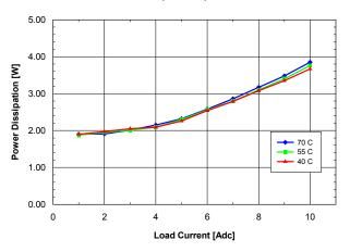
Figure 5. Power dissipation vs. load current and ambient temperature for SSQE48T10033 converter mounted vertically with Vin = 48 V and air flowing from pin 1 to pin 3at a rate of 200 LFM (1.0 m/s).
