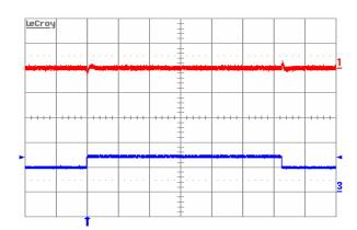
Figure 9. Output voltage response to load current stepchange (5A-7.5A-5A) at Vin=48V. Top trace: output voltage (100 mV/div.). Bottom trace: load current (5A/div.). Current slew rate: 5A/µs. Co= 470µF POS + 1µF ceramic. Time scale: 0.2 ms/div.
