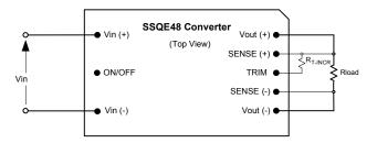
Fig. C: Configuration for increasing output voltage.
