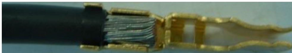
Picture 4 - Wire and Terminal before Crimping
