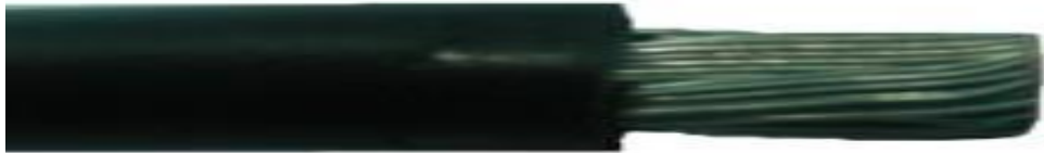
Picture 3 - The wire stripped
